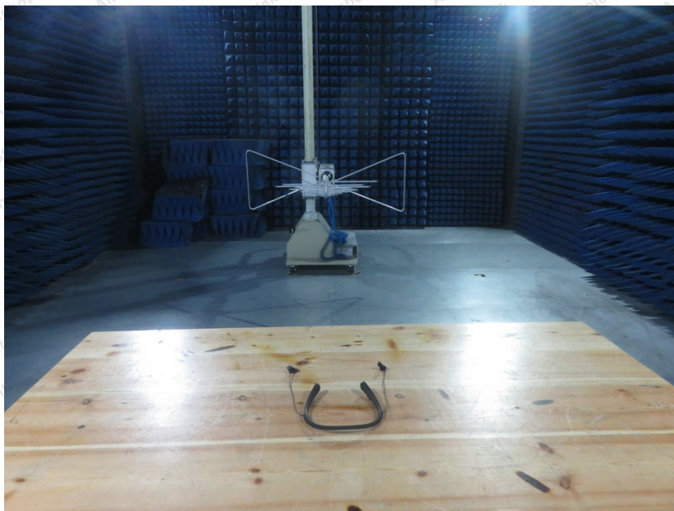
Photo of Radiation Emission Test
