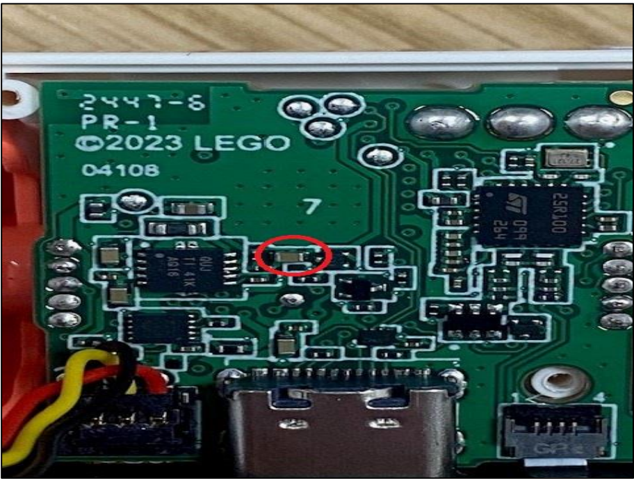
Figure 14 - Photograph showing the test point at which the voltage was measured to the RF Circuitry
