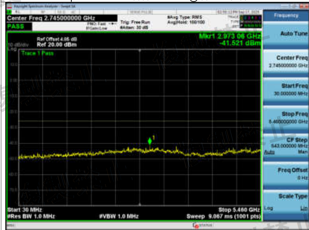
Tx. Spurious NVNT a 5600MHz Ant1 @ 5460MHz-5470MHz
