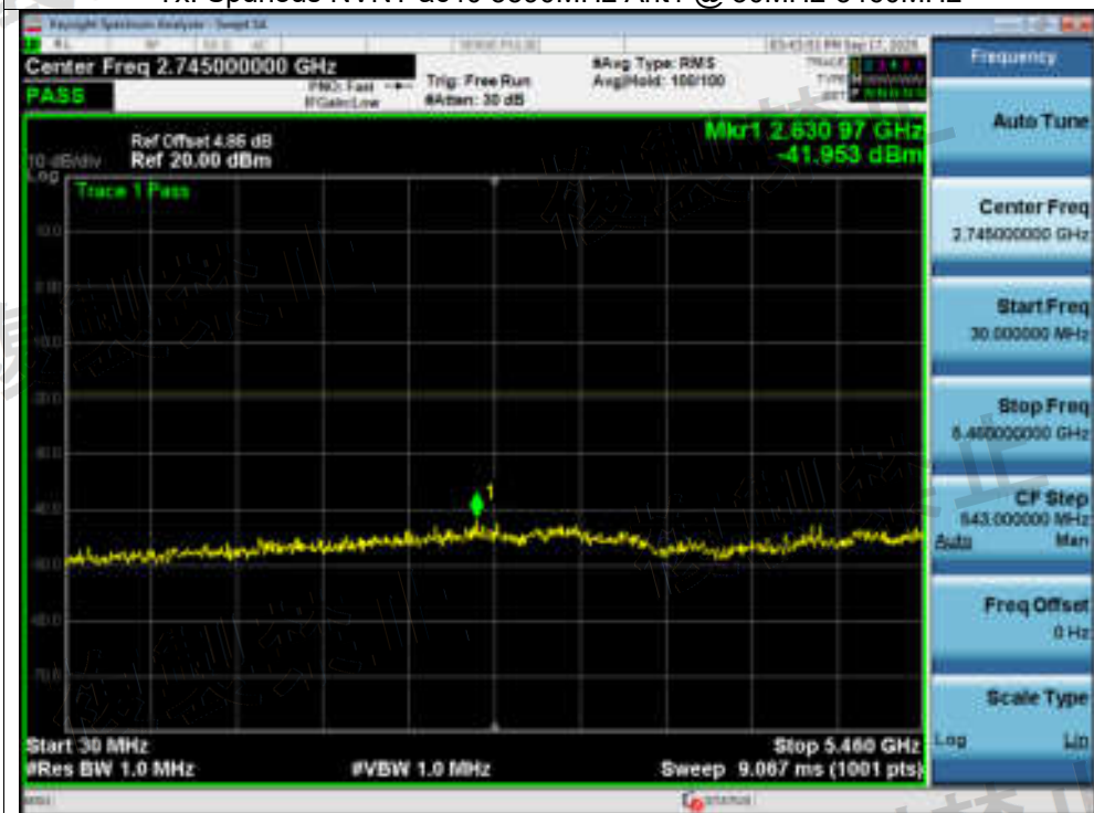
Tx. Spurious NVNT ac40 5590MHz Ant1 @ 5460MHz-5470MHz
