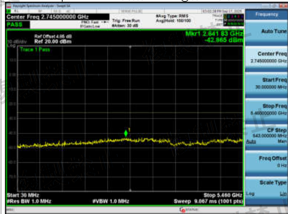
Tx. Spurious NVNT n20 5600MHz Ant1 @ 5460MHz-5470MHz
