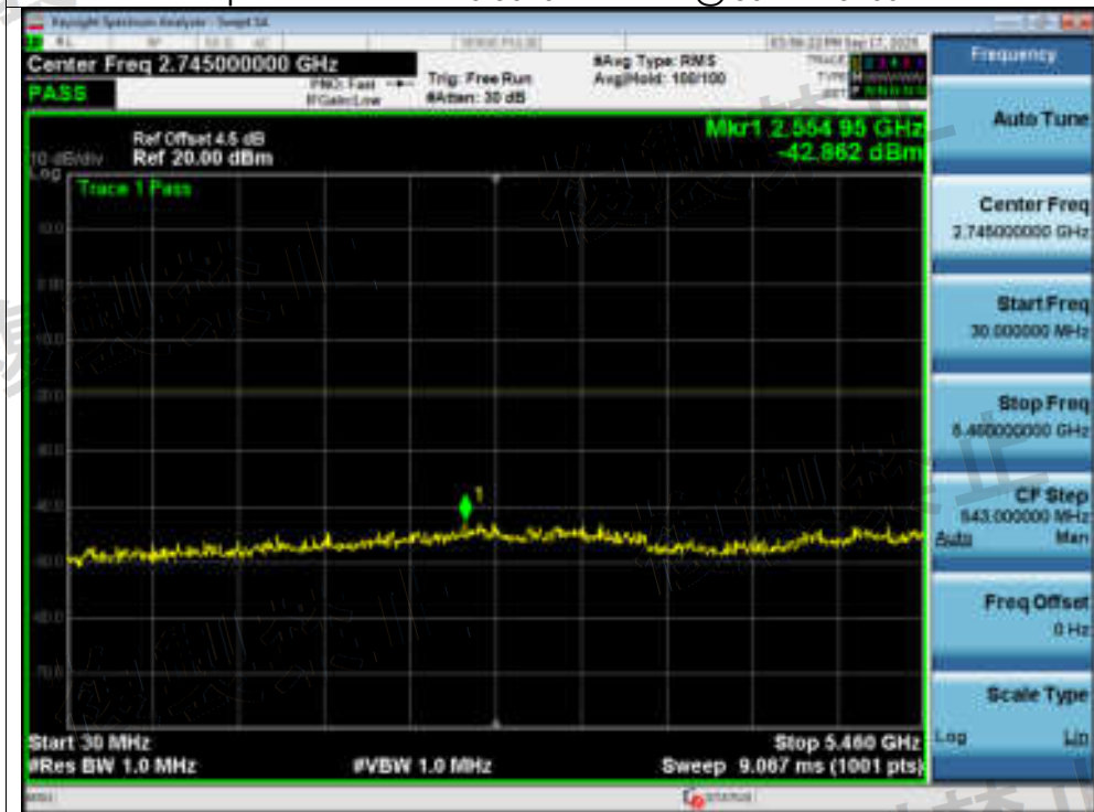
Tx. Spurious NVNT ax40 5670MHz Ant1 @ 5460MHz-5470MHz
