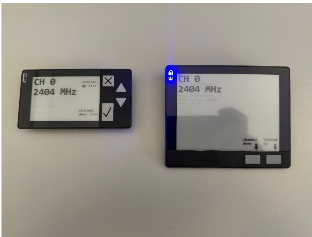
Photograph 15: Radio interference prevention capability test. The identification code is the predetermined one. Communication is normal (light is blue).
