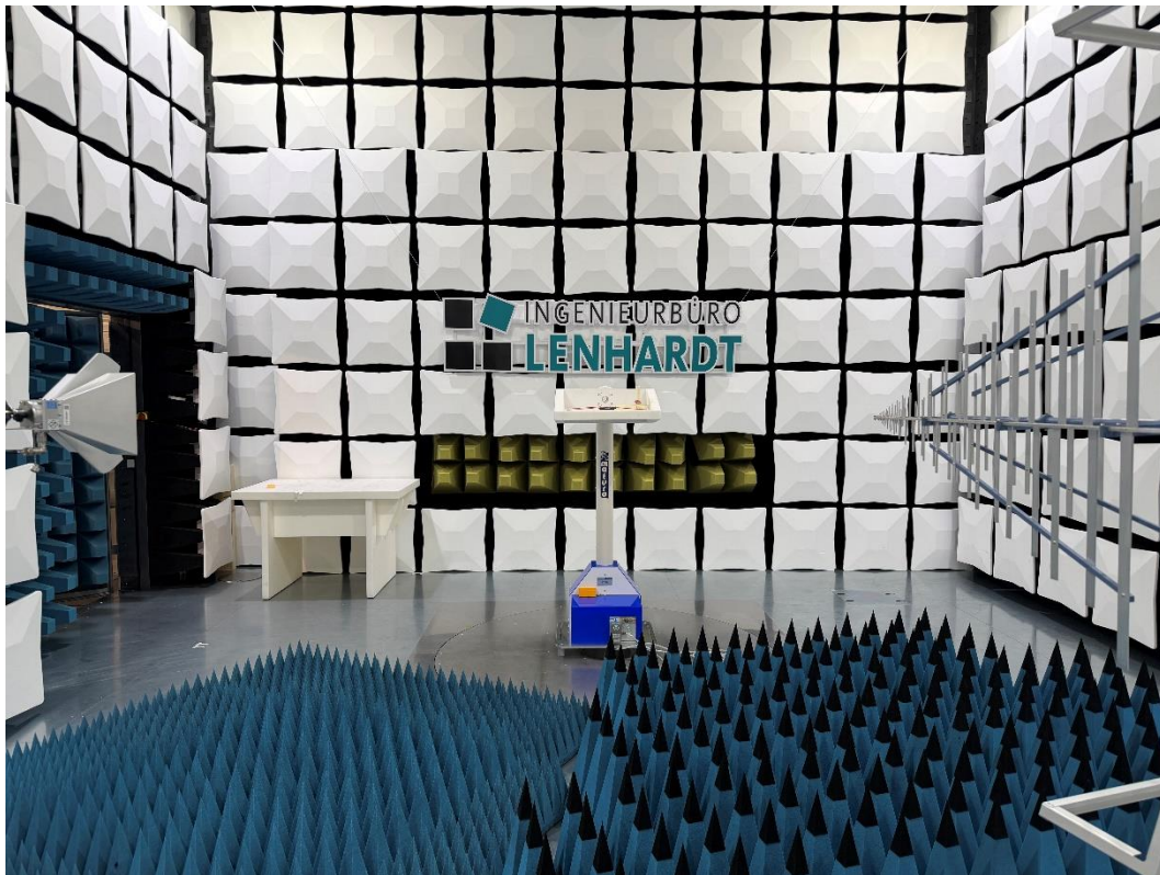
Photograph 13: Measurement set-up radiated, overall view.
