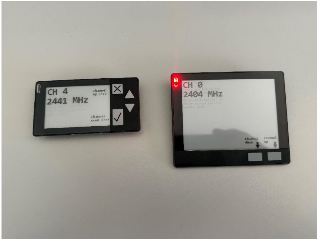
Photograph 16: Radio interference prevention capability test. The light is red, what means, that the identification code is different from the predetermined one.
