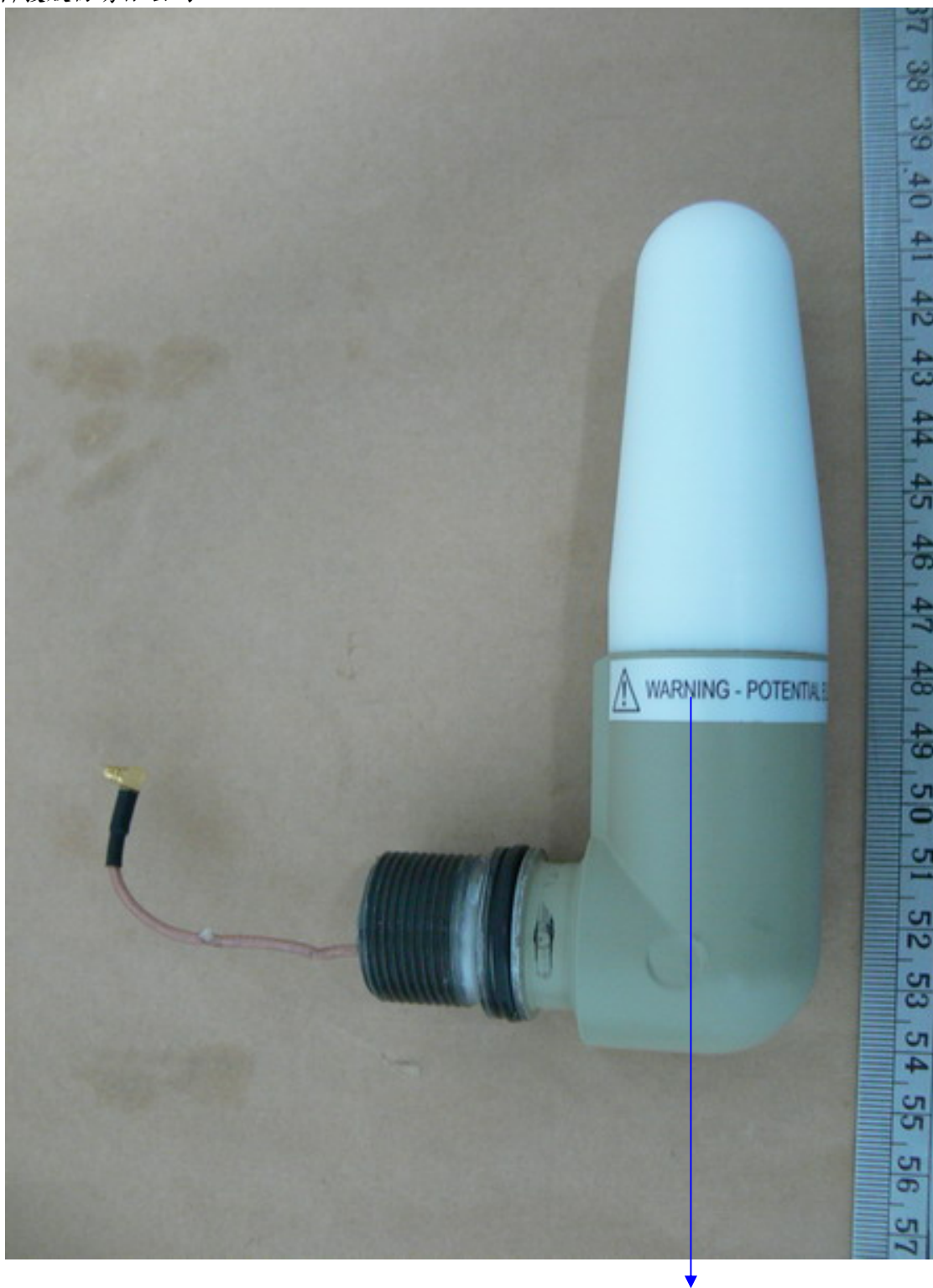
Integral antenna (廠牌：CENTURION，型號：MAF94152) Antenna gain: -2 dBi
