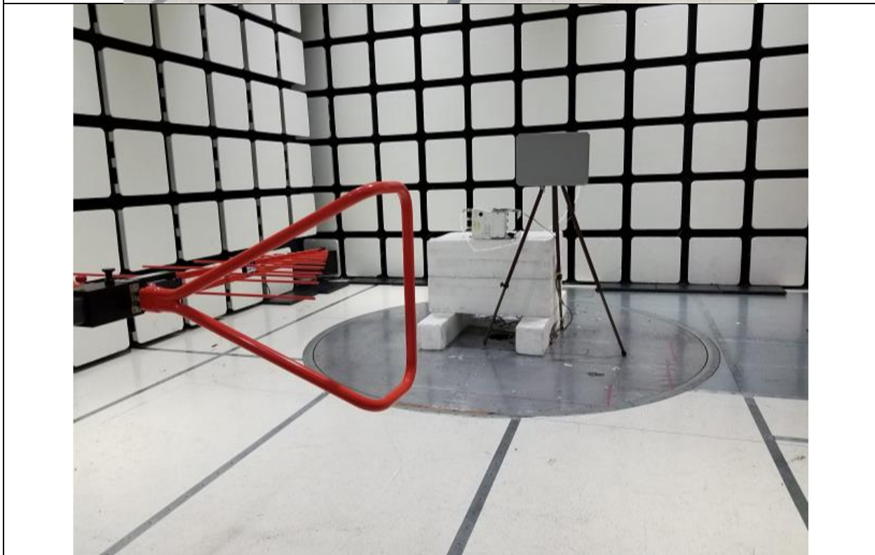
Title: Radiated Spurious Emissions 30MHz-1GHz – Test Setup
