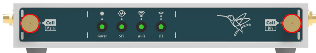
Fig. 20: WWAN Main and Div antenna connectors
