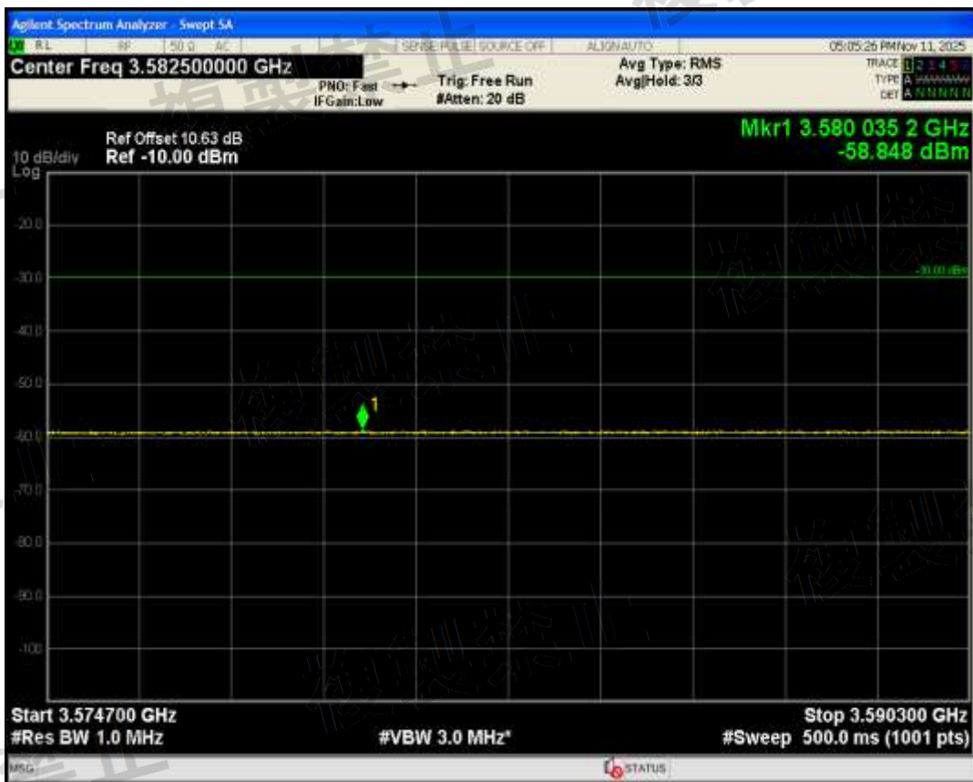
Band1(5L) QPSK BW=5MHz Channel=18025 RB Size=1 Position=#0 Range3590.3 MHz-3600 MHz
