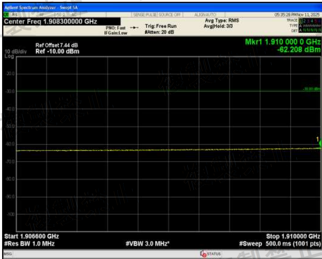
Band1(5L) QAM16 BW=5MHz Channel=18046 RB Size=25 Position=#0 Range1910 MHz-1915.7 MHz
