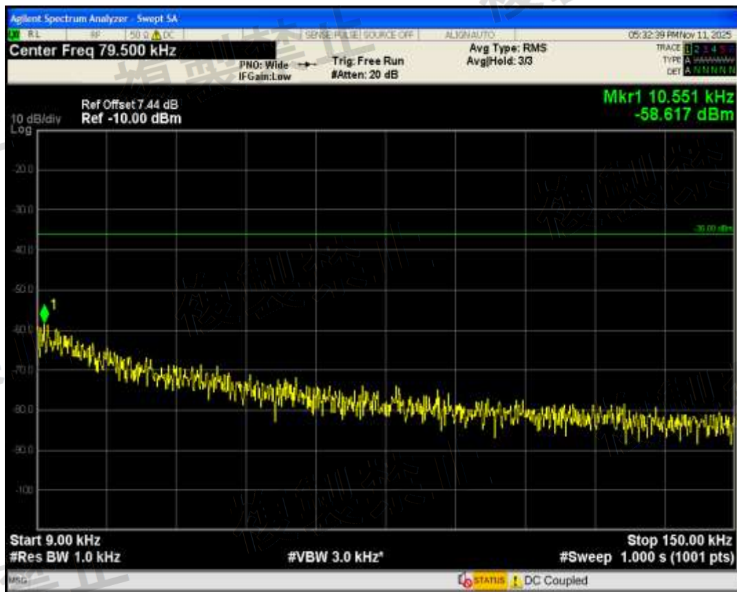
Band1(5L) QAM16 BW=5MHz Channel=18046 RB Size=1 Position=#Max Range150 kHz-30 MHz
