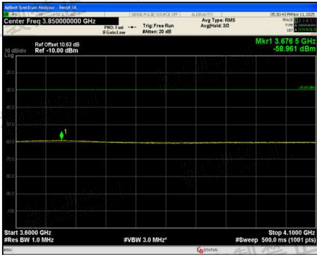
Band1(5L) QPSK BW=5MHz Channel=18046 RB Size=25 Position=#0 Range3590.3 MHz-3600 MHz
