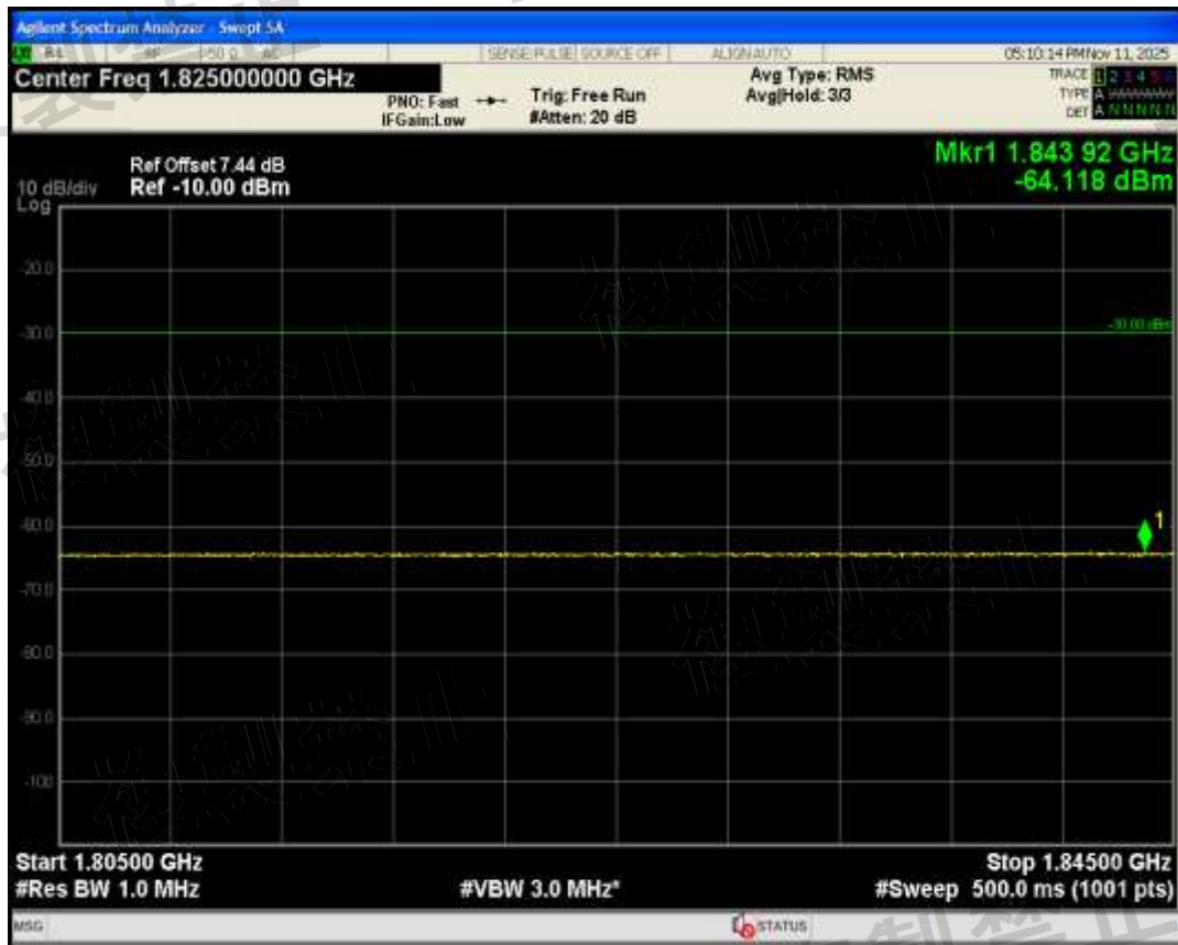
Band1(5L) QAM16 BW=5MHz Channel=18025 RB Size=1 Position=#0 Range1845 MHz-1880 MHz
