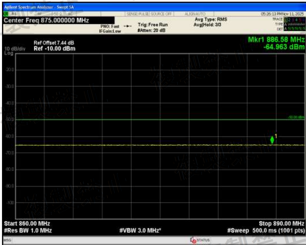
Band1(5L) QPSK BW=5MHz Channel=18046 RB Size=1 Position=#0 Range945 MHz-960 MHz
