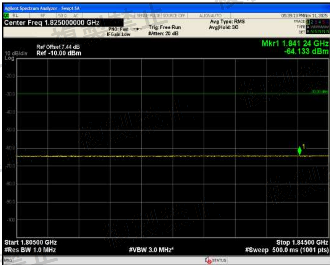
Band1(5L) QPSK BW=5MHz Channel=18046 RB Size=1 Position=#Max Range1496.6 MHz-1510.9 MHz
