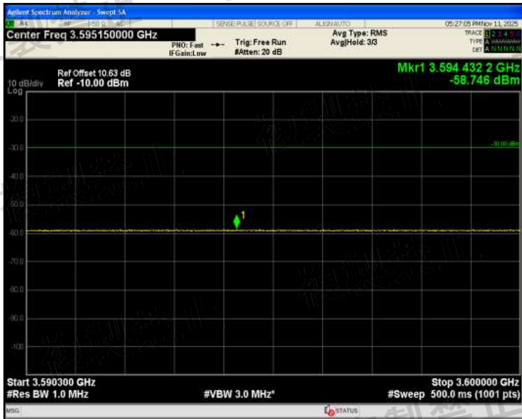
Band1(5L) QPSK BW=5MHz Channel=18046 RB Size=1 Position=#0 Range3600 MHz-4100 MHz
