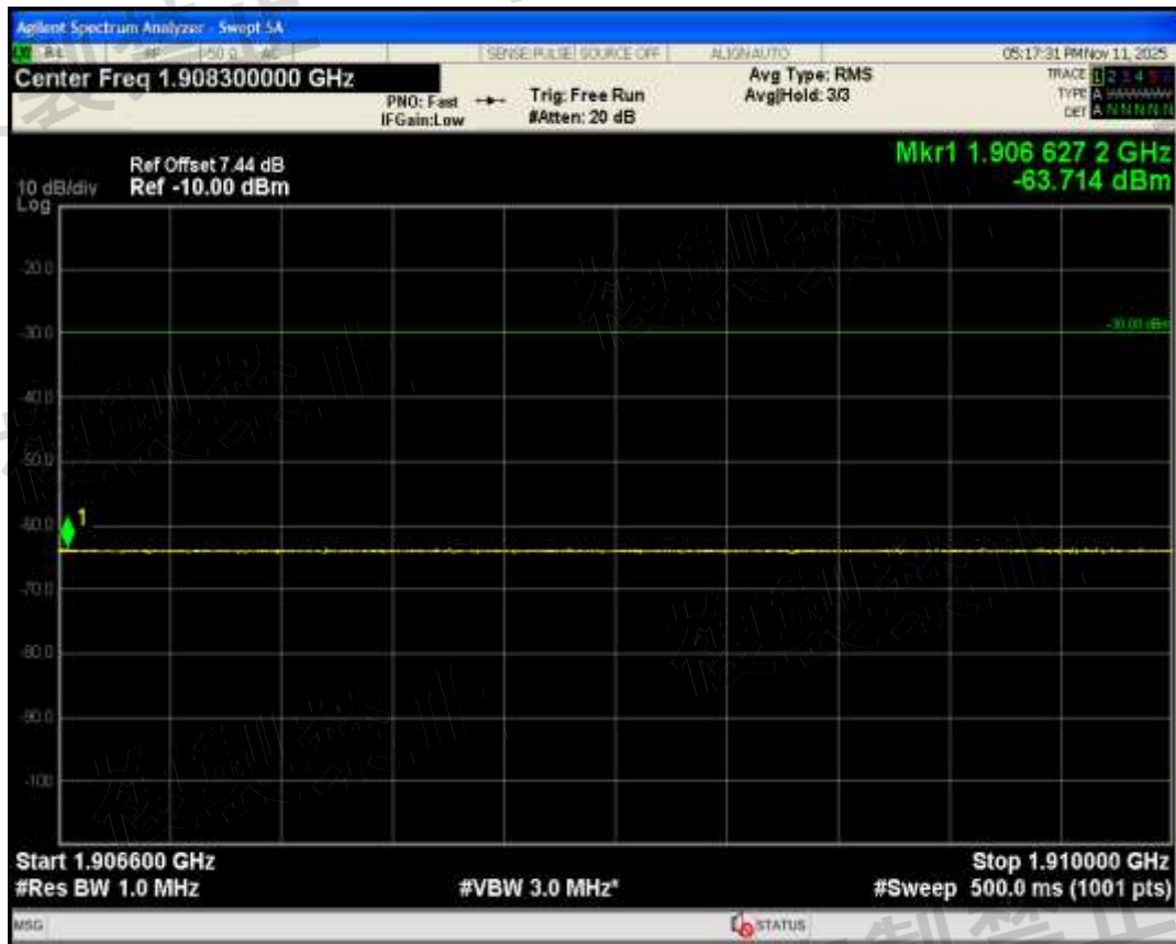
Band1(5L) QPSK BW=5MHz Channel=18036 RB Size=1 Position=#Max Range2010 MHz-2025 MHz
