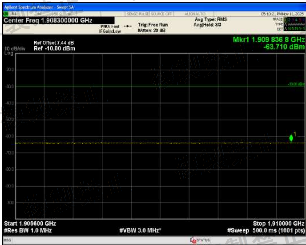
Band1(5L) QAM16 BW=5MHz Channel=18025 RB Size=1 Position=#0 Range1910 MHz-1915.7 MHz
