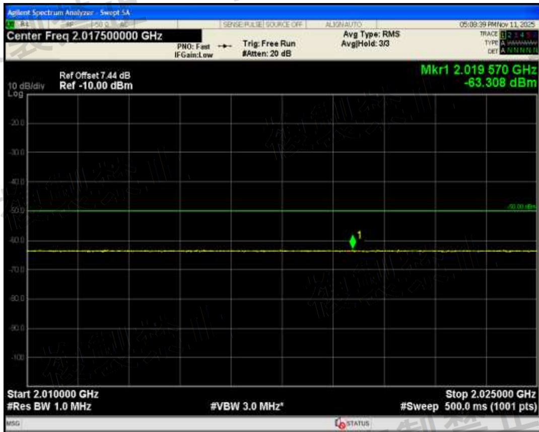
Band1(5L) QPSK BW=5MHz Channel=18025 RB Size=25 Position=#0 Range2144.4 MHz-2170 MHz
