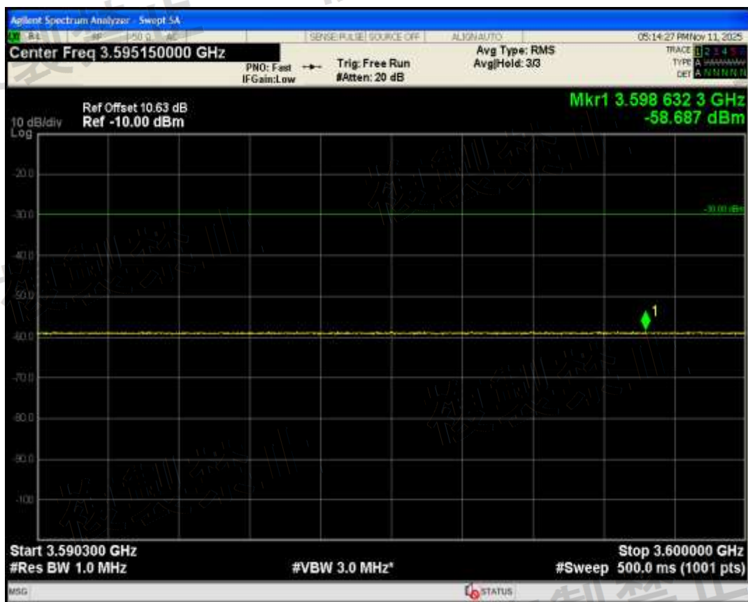
Band1(5L) QAM16 BW=5MHz Channel=18025 RB Size=25 Position=#0 Range3600 MHz-4100 MHz
