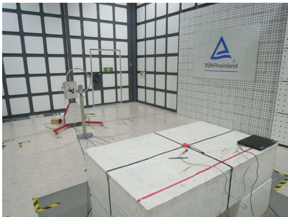
Photograph 5: Set-up for Spurious Emissions (Back View 3)
