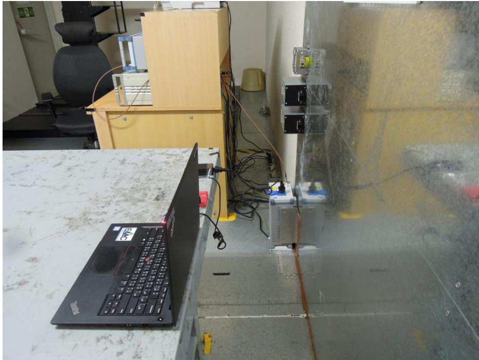
Photograph 9: Set-up for Mains Conducted testing (Front View)
