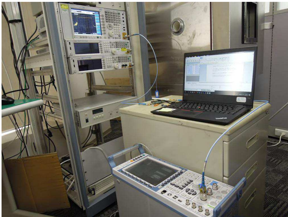
Photograph 7: Set-up for Conducted testing
