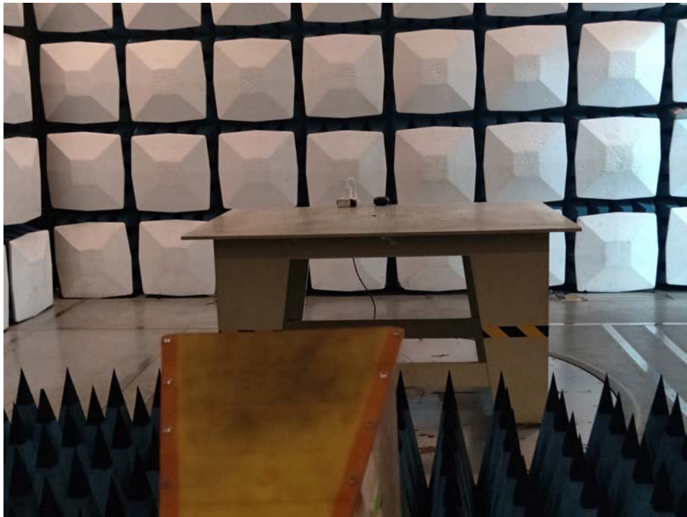
Radiated Emission Above 1G -rear View
