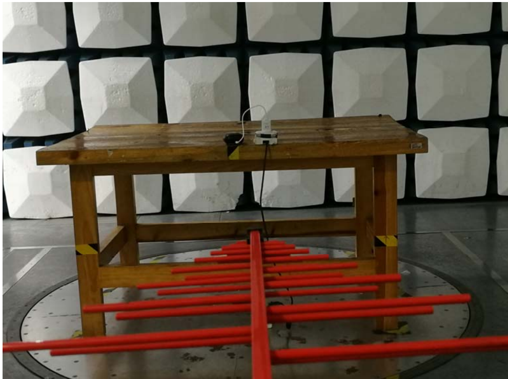
Radiated Emission Below 1G -rear View
