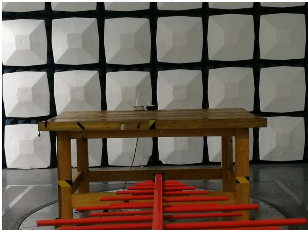
Radiated Emission Below 1G -rear View
