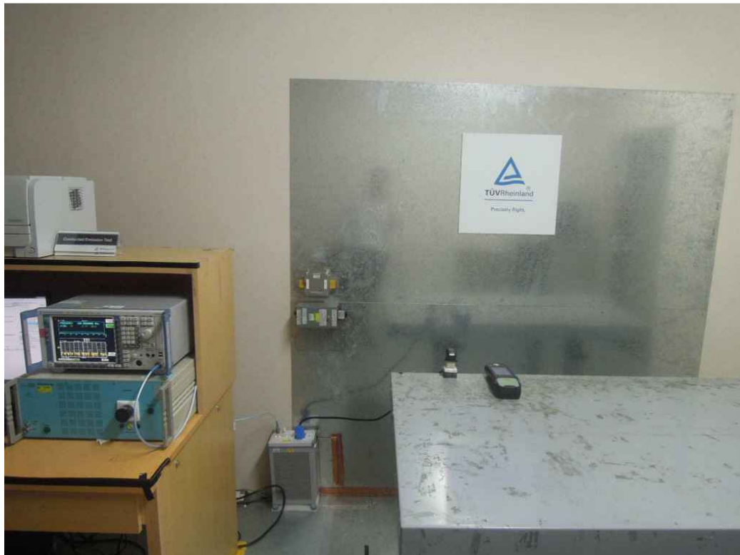
Photograph 10: Set-up for Mains Conducted testing Front
