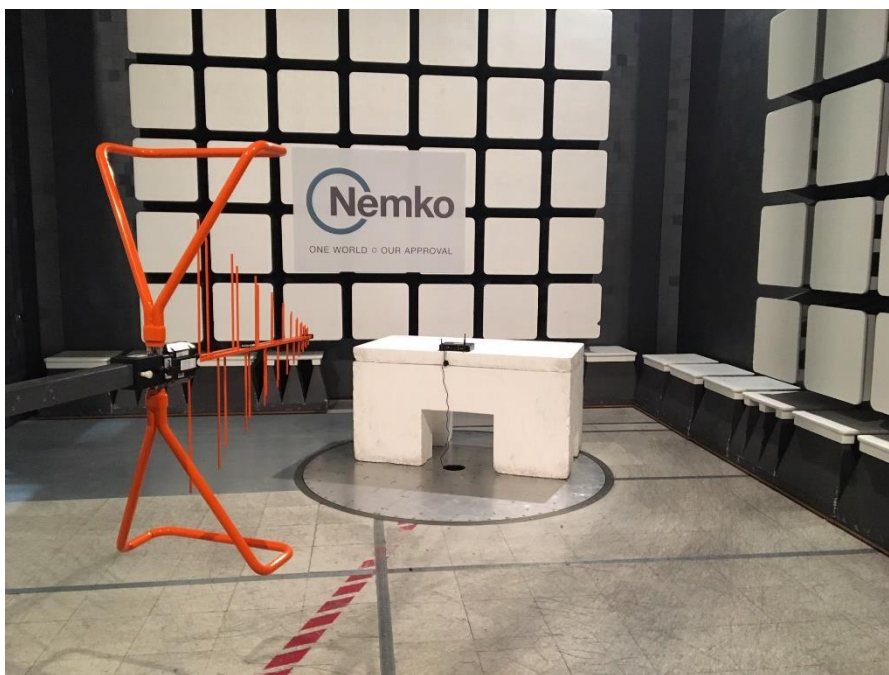
Figure 8.3-30: Radiated spurious emissions setup photo – below 1 GHz
