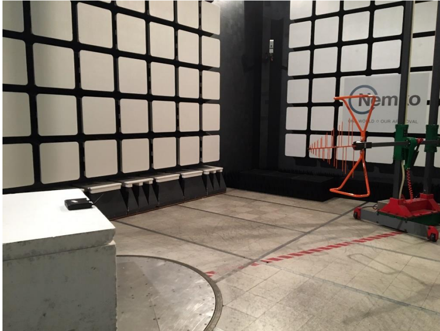
Figure 8.3-29: Radiated spurious emissions setup photo – below 1 GHz
