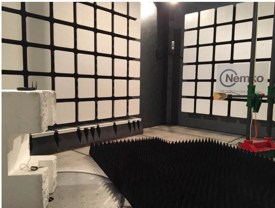
Figure 8.3-32: Radiated spurious emissions setup photo – above 1 GHz
