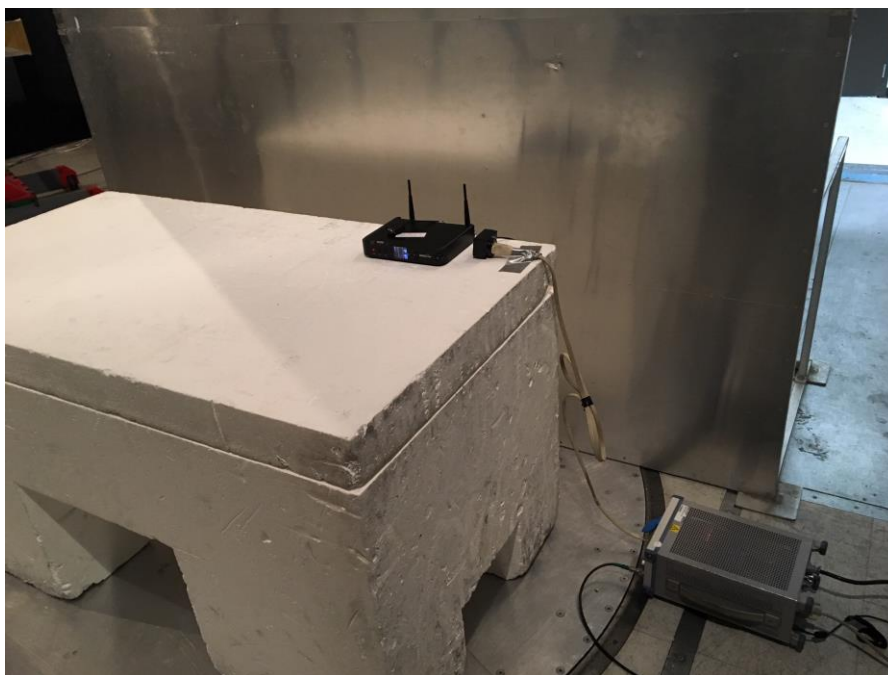
Figure 8.5-3: Conducted emissions – from AC mains power ports setup photo
