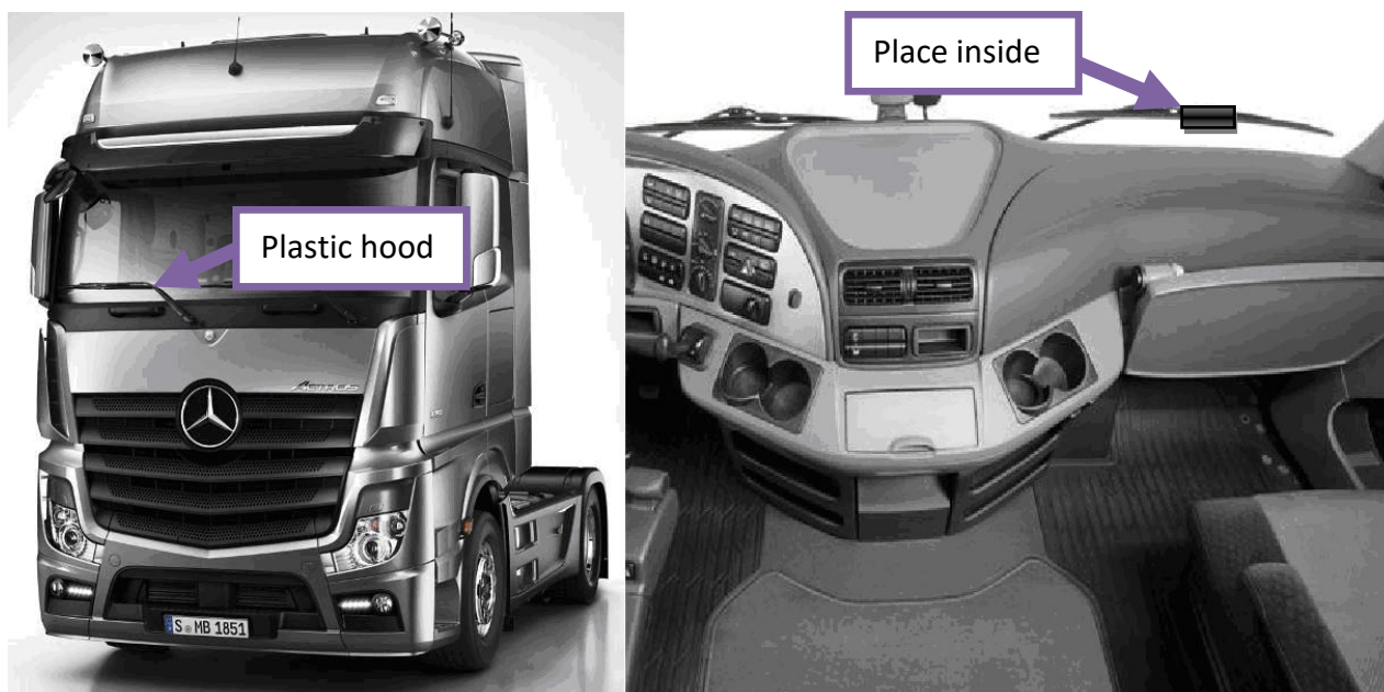
Figure 58. Possible mounting places in trucks
