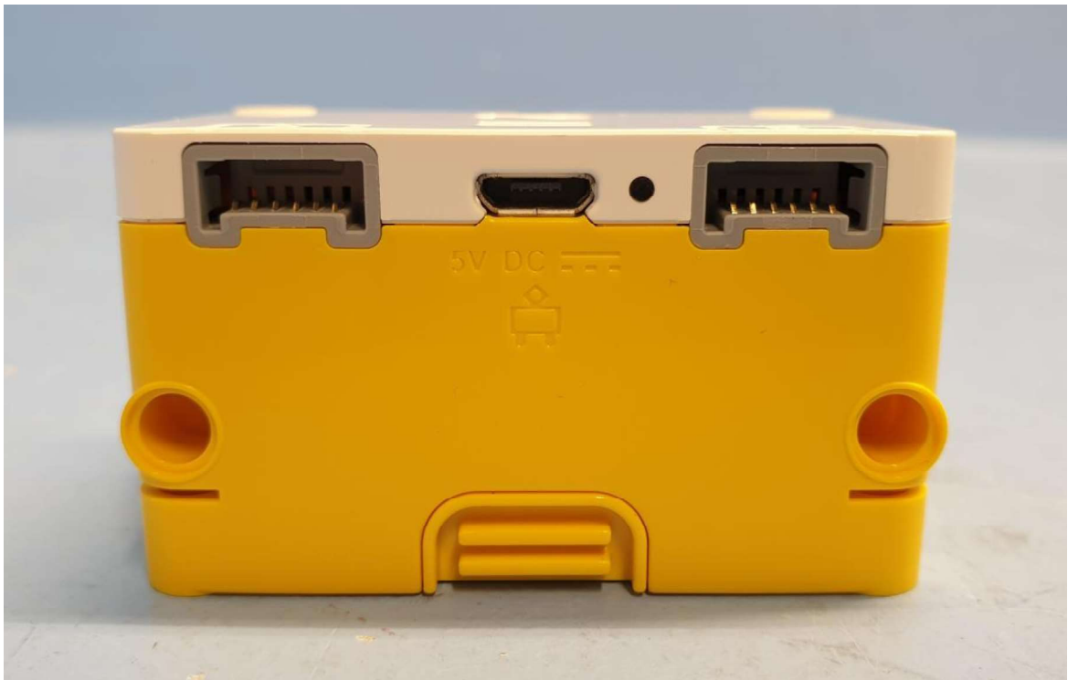
Side view, USB connector and LFP2 ports
