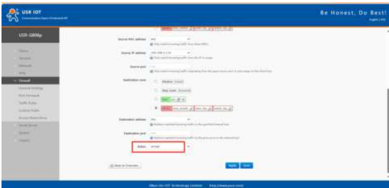
Pic 59 Figure 3: Firewall whitelist
