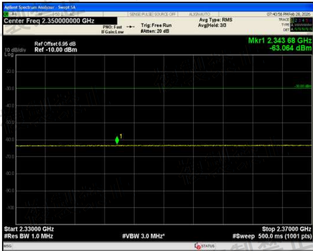
Band1(15H) QAM16 BW=15MHz Channel=18411 RB Size=75 Position=#0 Range2144.4 MHz-2170 MHz
