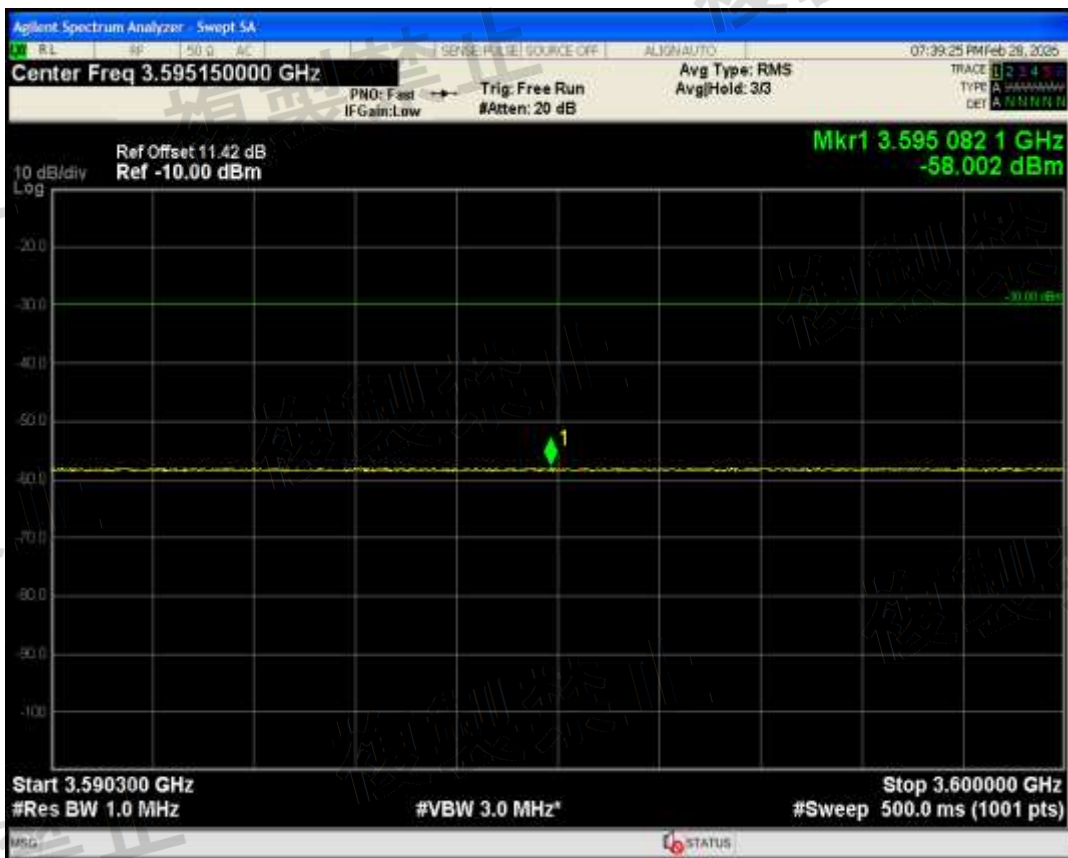
Band1(15H) QAM16 BW=15MHz Channel=18411 RB Size=1 Position=#Max Range3574.7 MHz-3590.3 MHz
