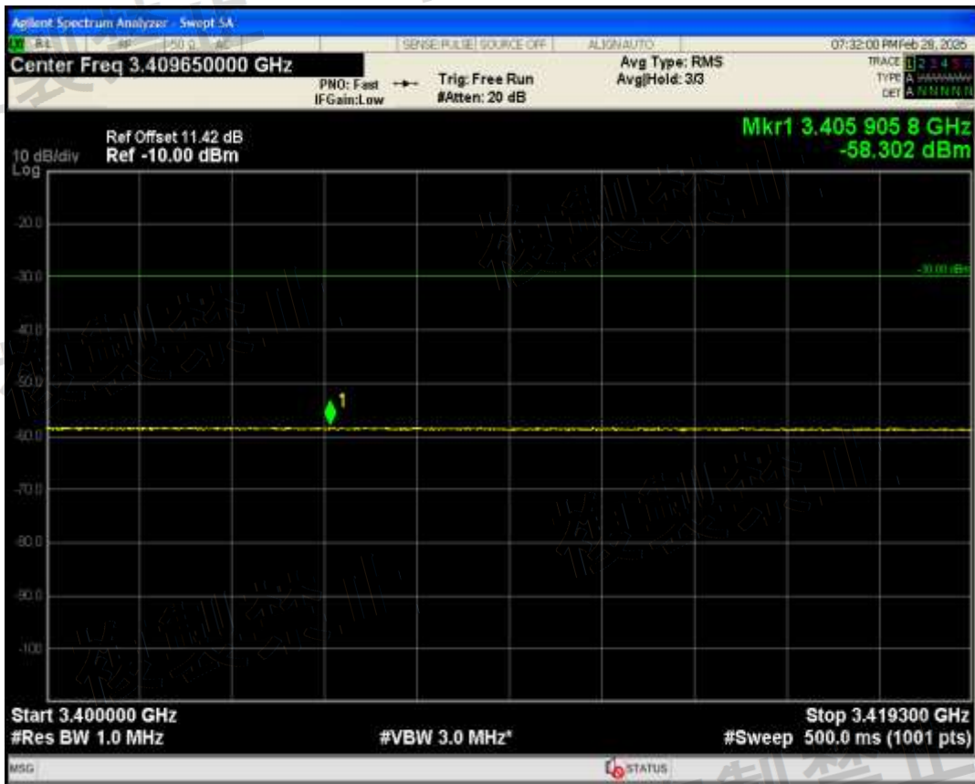
Band1(15H) QPSK BW=15MHz Channel=18411 RB Size=1 Position=#0 Range3419.3 MHz-3500.7 MHz
