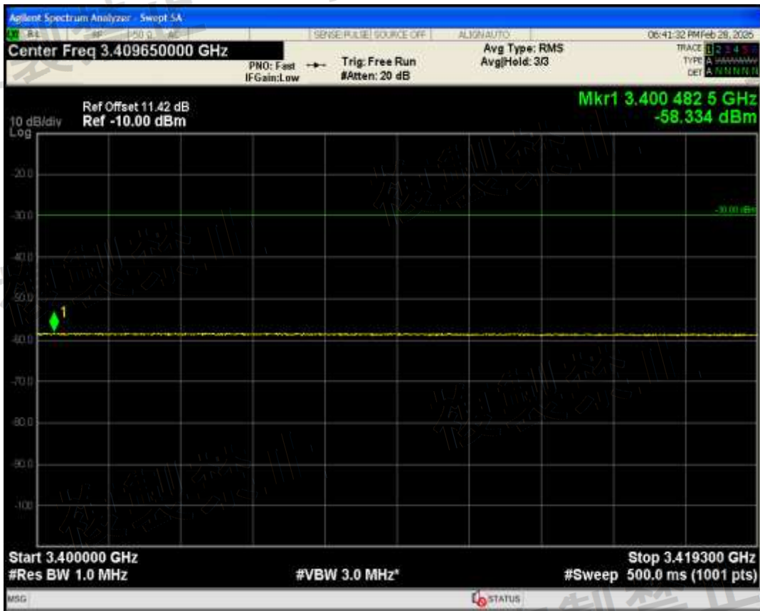
Band1(15L) QPSK BW=15MHz Channel=18075 RB Size=1 Position=#Max Range3419.3 MHz-3500.7 MHz
