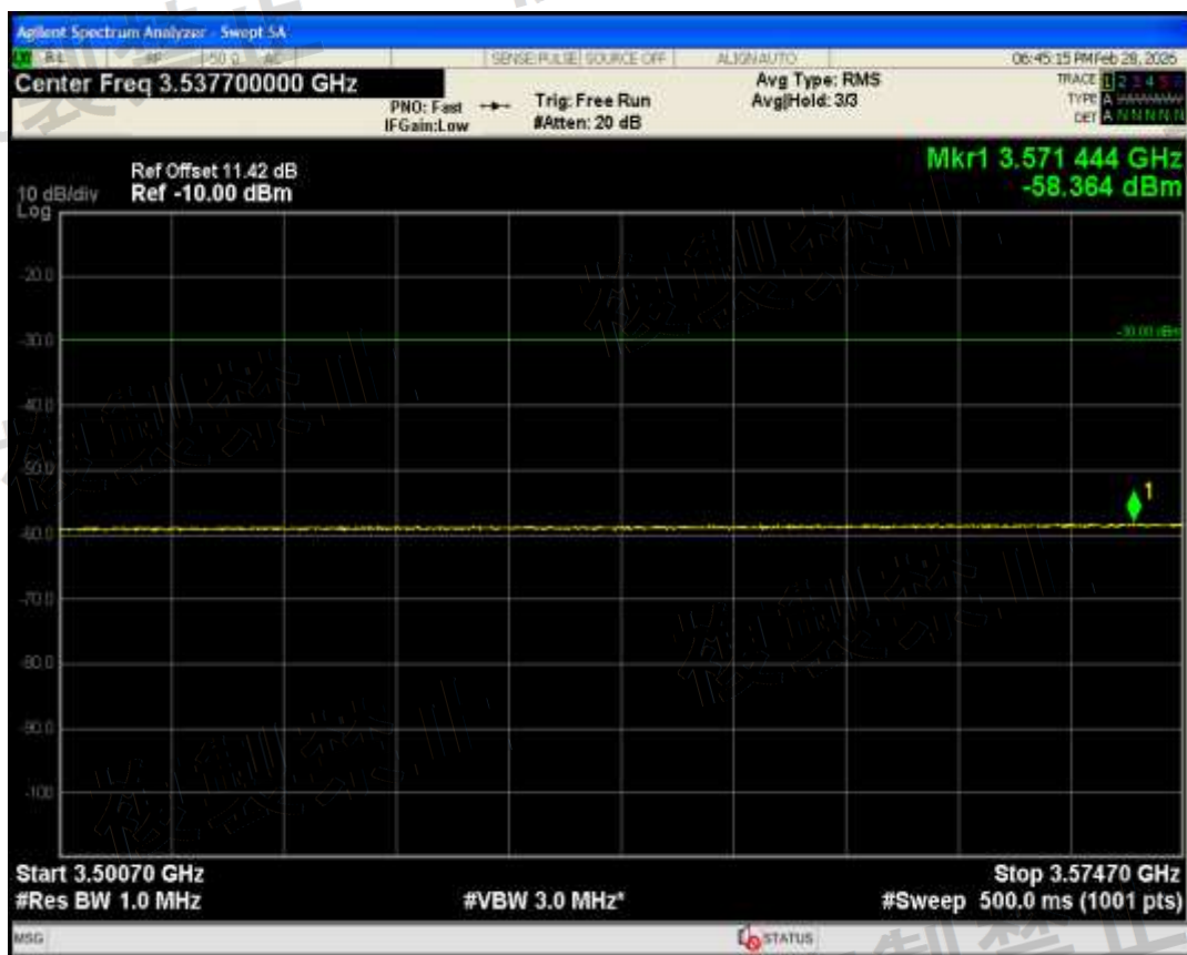
Band1(15L) QAM16 BW=15MHz Channel=18075 RB Size=1 Position=#0 Range3574.7 MHz-3590.3 MHz
