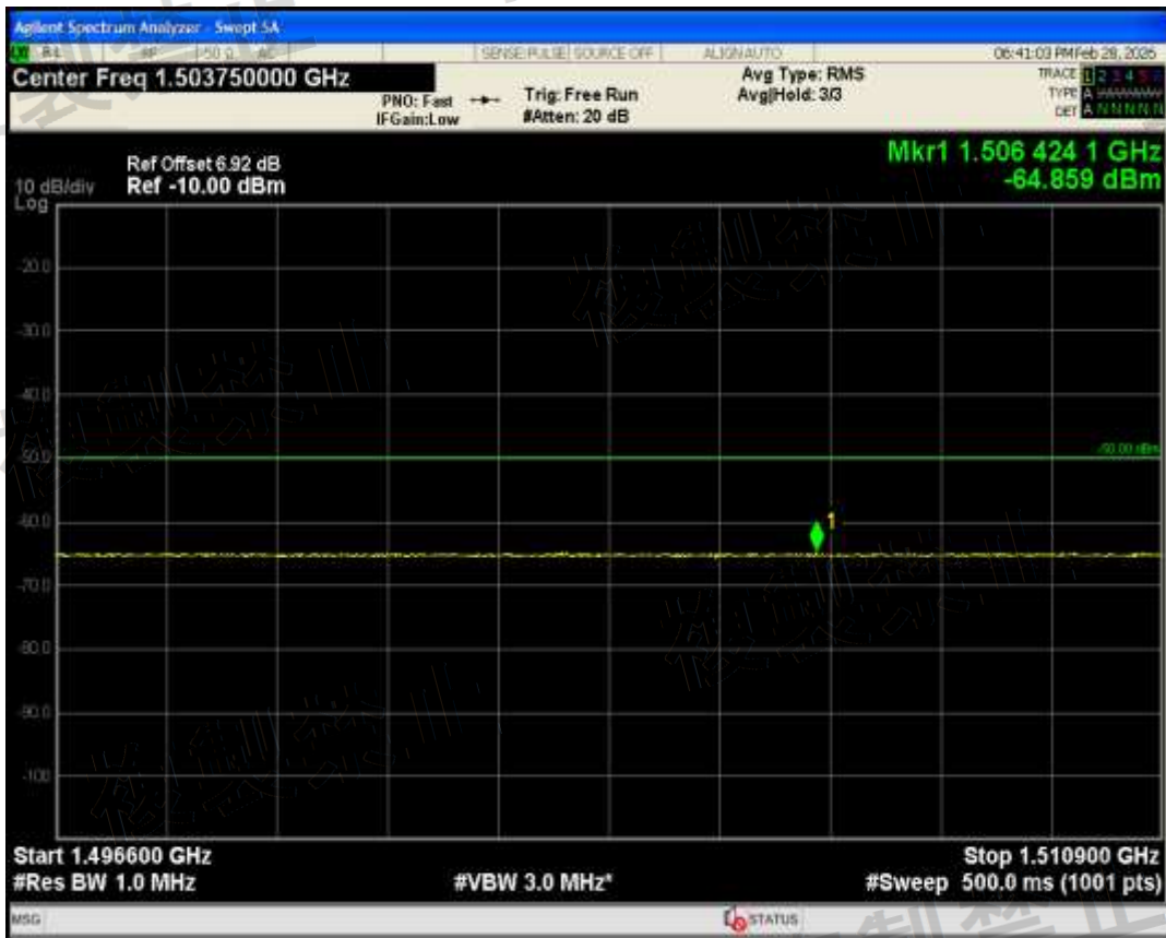
Band1(15L) QPSK BW=15MHz Channel=18075 RB Size=1 Position=#Max Range1475.9 MHz-1496.6 MHz
