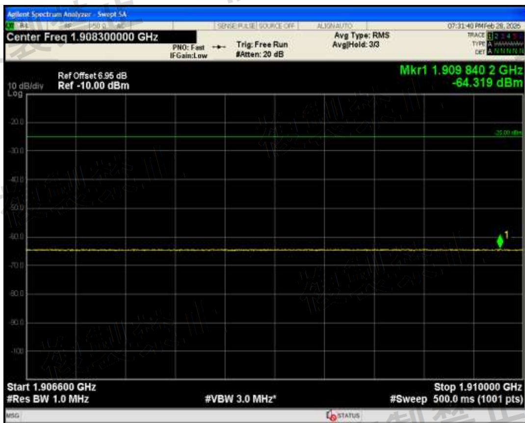
Band1(15H) QPSK BW=15MHz Channel=18411 RB Size=1 Position=#0 Range1910 MHz-1915.7 MHz
