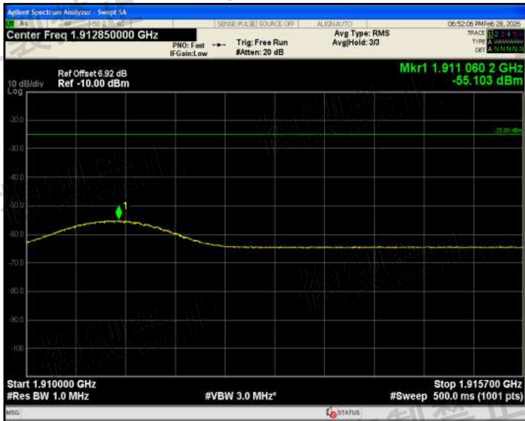
Band1(15L) QPSK BW=15MHz Channel=18110 RB Size=1 Position=#Max Range1906.6 MHz-1910 MHz
