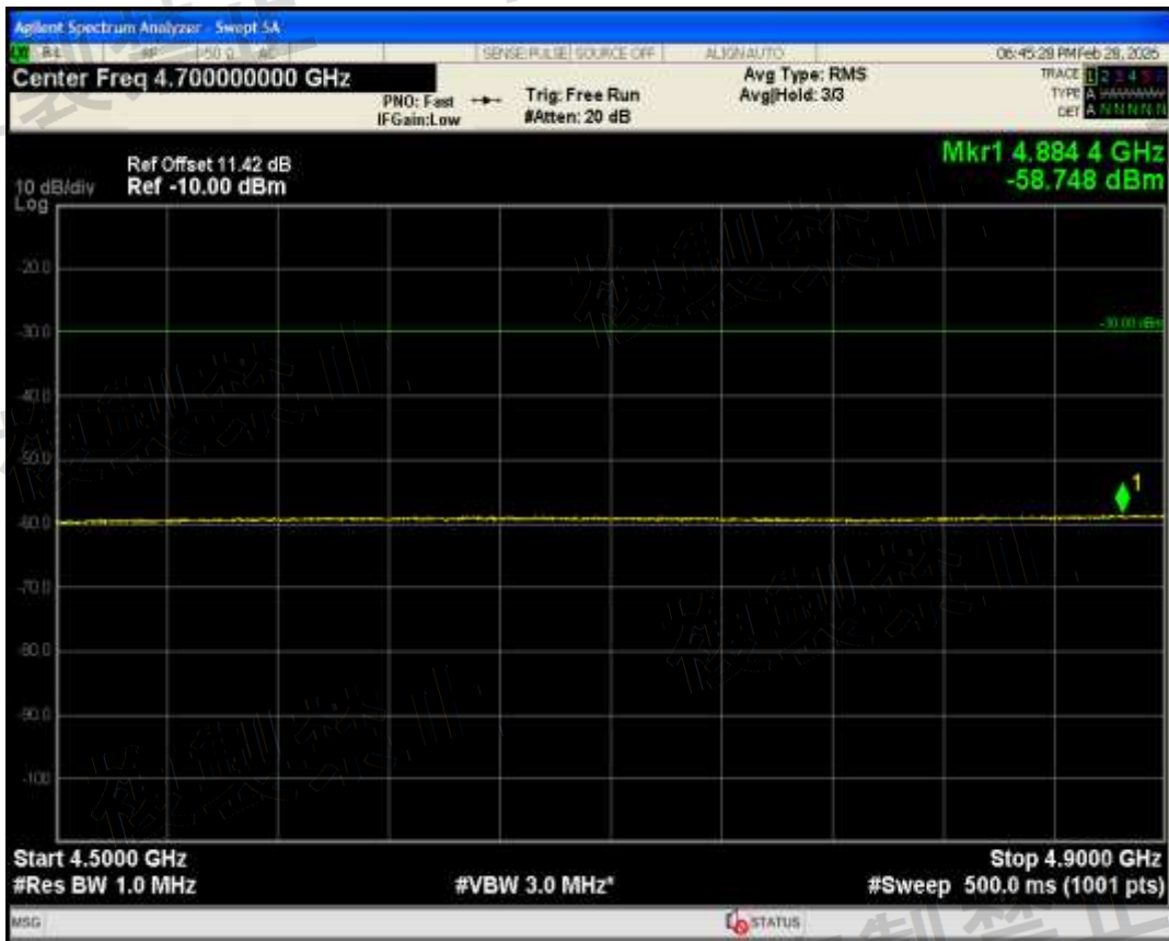
Band1(15L) QAM16 BW=15MHz Channel=18075 RB Size=1 Position=#Max Range9 kHz-150 kHz
