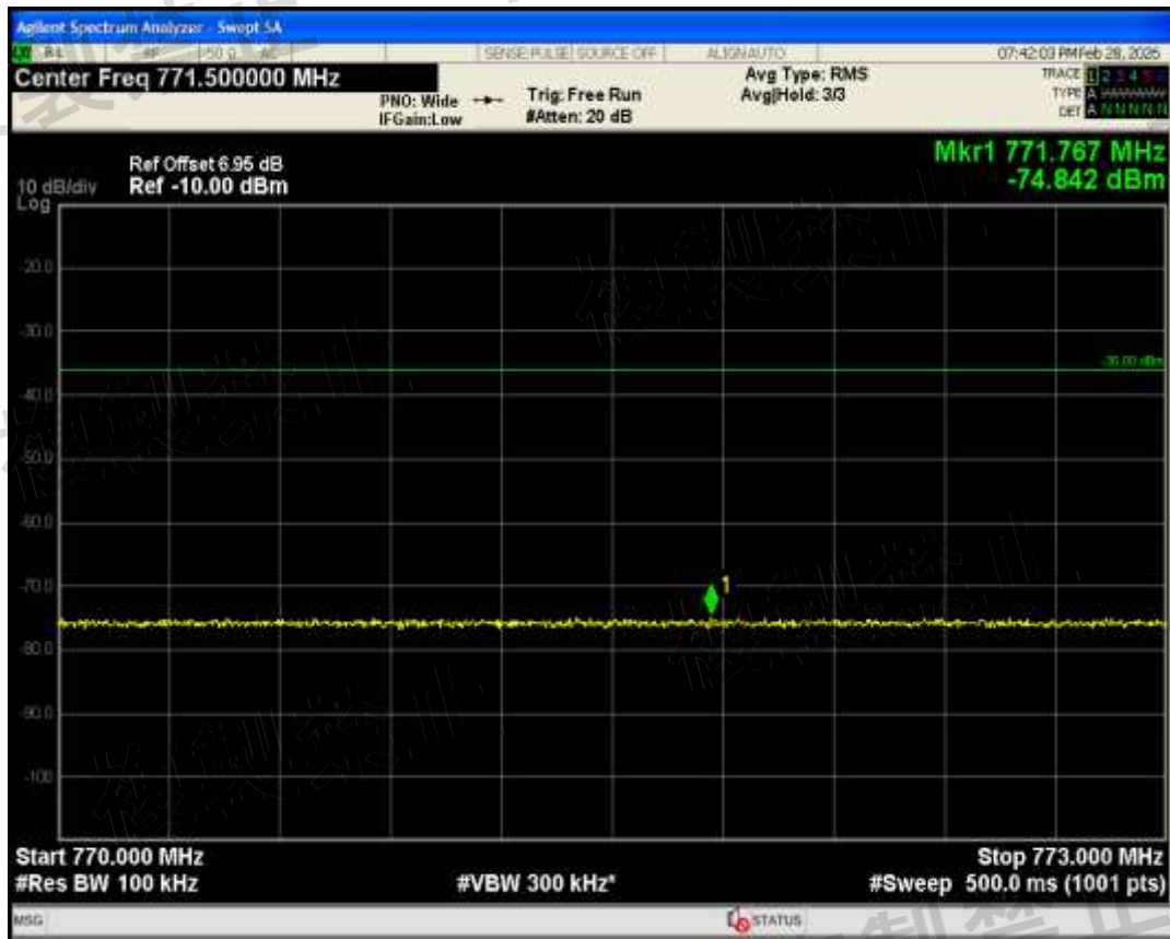
Band1(15H) QPSK BW=15MHz Channel=18525 RB Size=1 Position=#0 Range773 MHz-803 MHz
