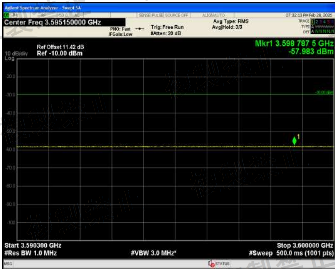
Band1(15H) QPSK BW=15MHz Channel=18411 RB Size=1 Position=#0 Range3600 MHz-4100 MHz
