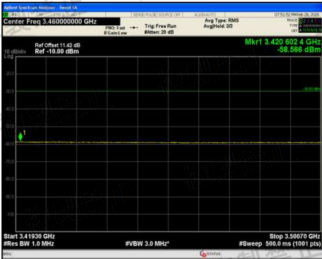
Band1(15H) QAM16 BW=15MHz Channel=18525 RB Size=75 Position=#0 Range3400 MHz-3419.3 MHz
