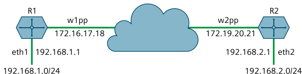
Figure 12.6 Example – GRE Tunnel Configuration
