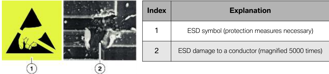
Effects of ESD (Electrostatic Discharge) on electronic components
