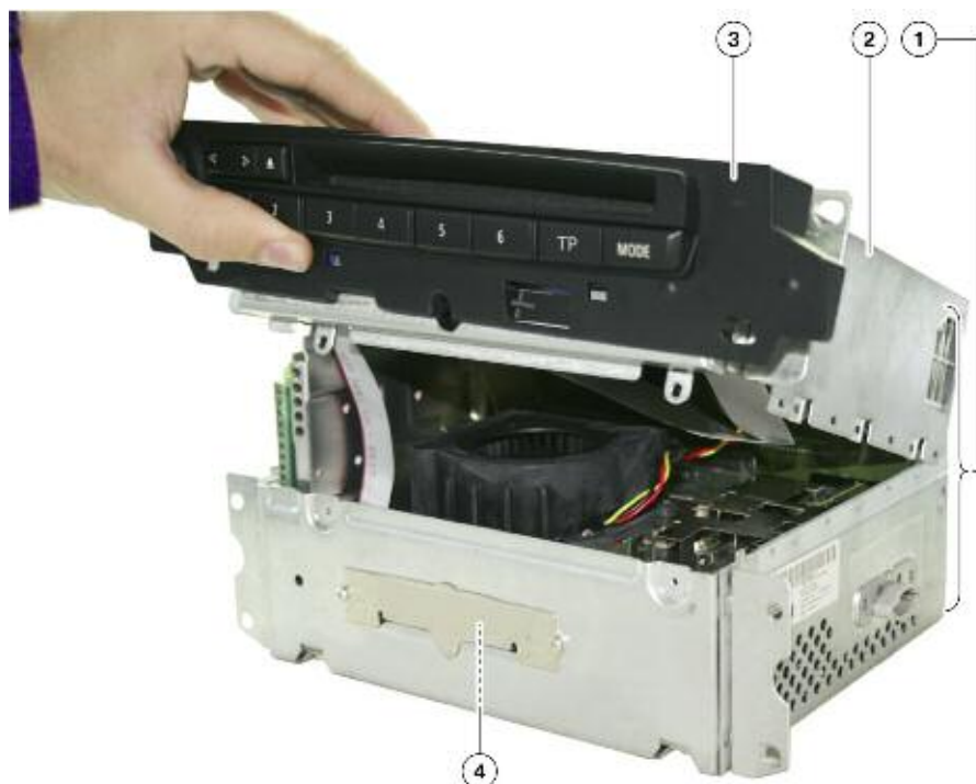
Individual replaceable components of the Car Information Computer
