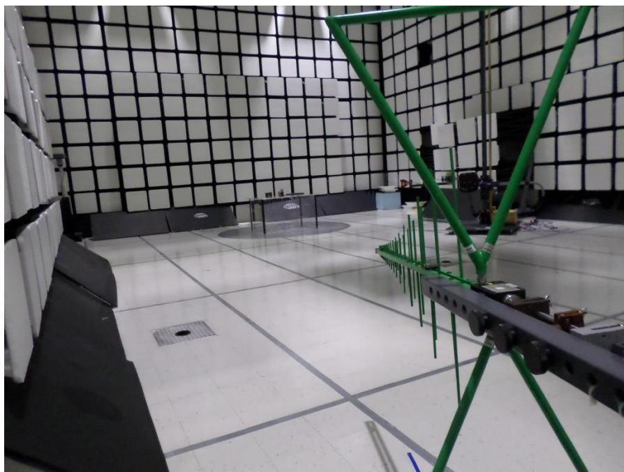
Figure 21. Spurious Emissions, Outside 13.56 MHz, Bilog Antenna View
