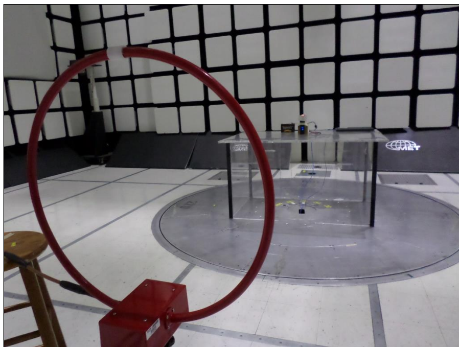
Figure 11. Emissions Within the Band 13.11 – 14.01 MHz, Loop Antenna View
