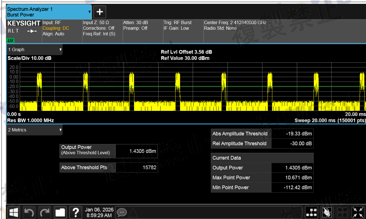
Power NVNT ax20 2442MHz Ant1 Pre Scan
