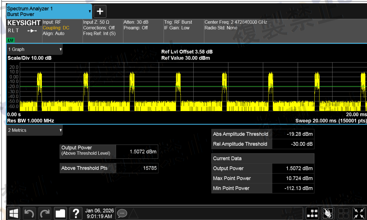
Power NVNT ax40 2422MHz Ant1 Pre Scan
