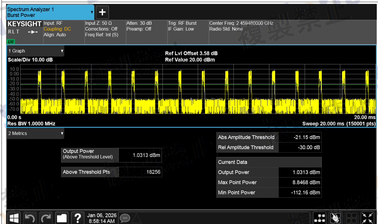
Power NVNT ax20 2412MHz Ant1 Pre Scan
