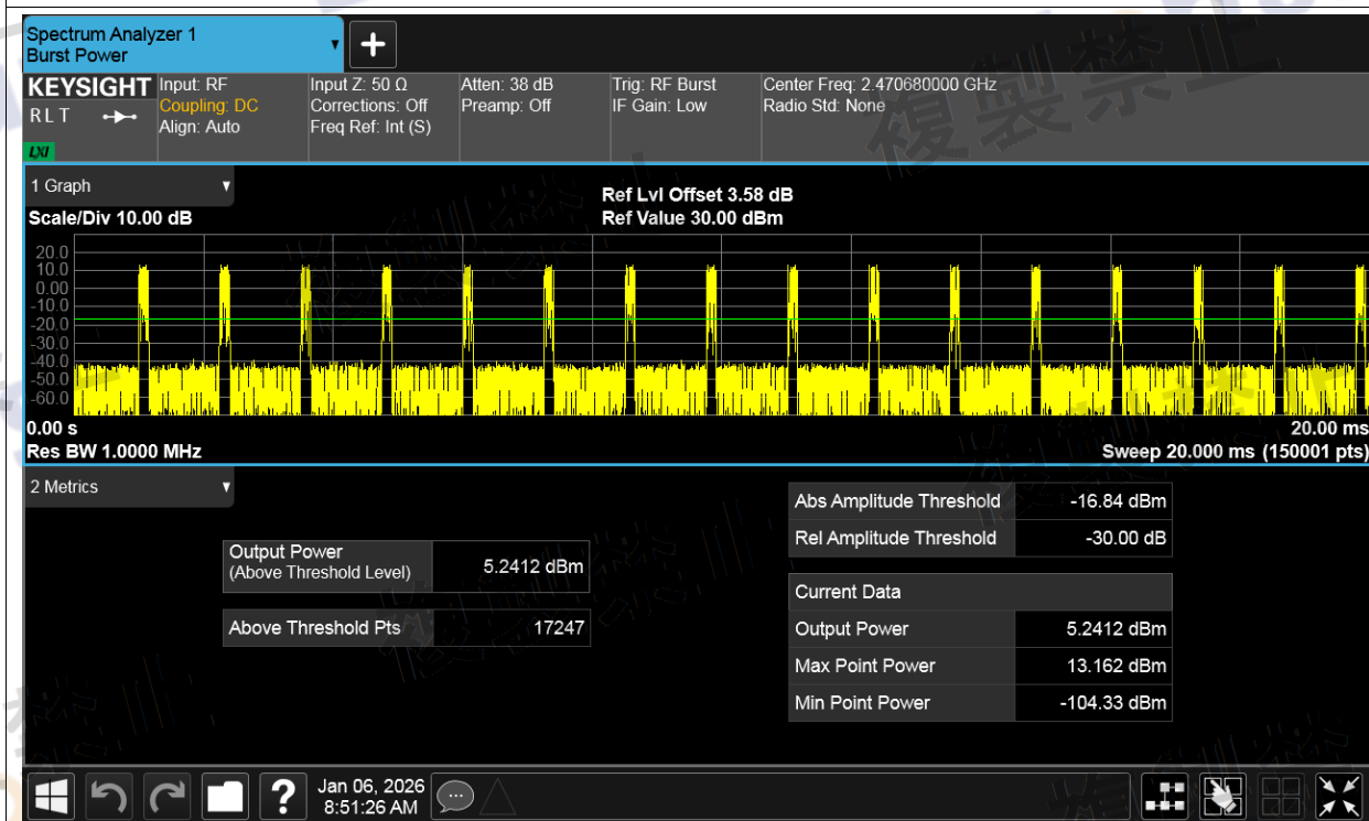
Power NVNT n20 2412MHz Ant1 Pre Scan
