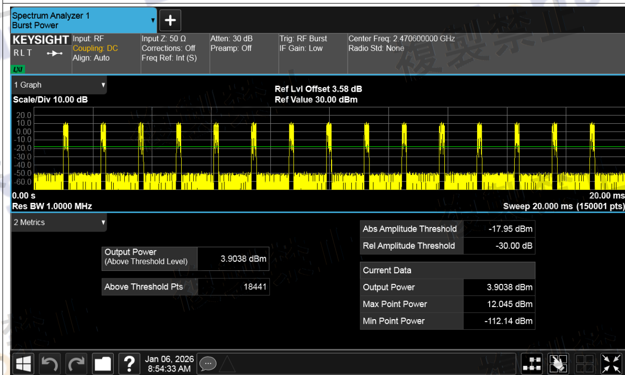
Power NVNT n40 2422MHz Ant1 Pre Scan
