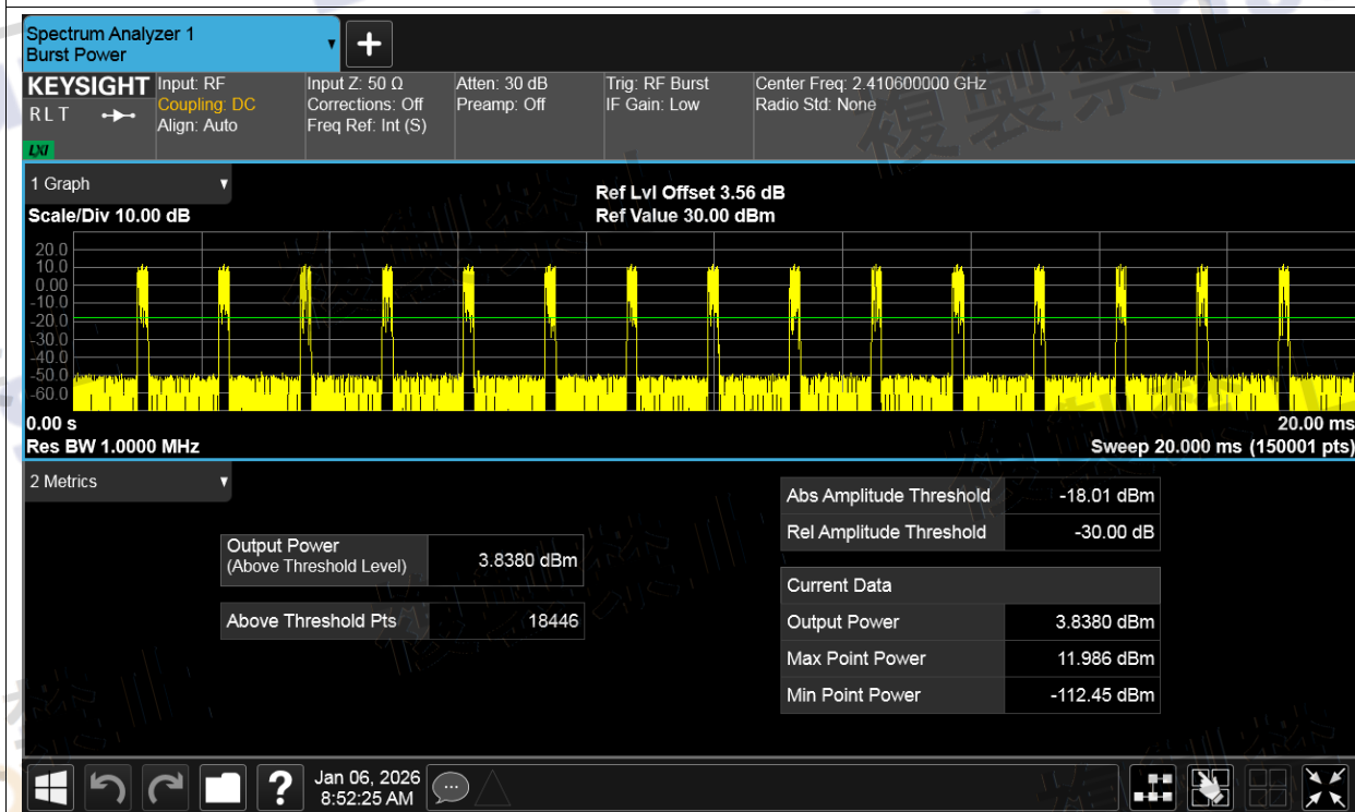
Power NVNT n20 2442MHz Ant1 Pre Scan
