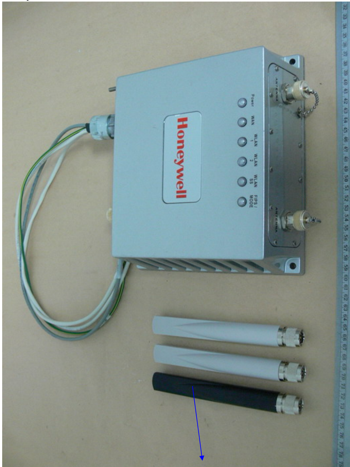
Portable Omni-Directional Antenna for FHSS part 天線增益:5 dBi。
