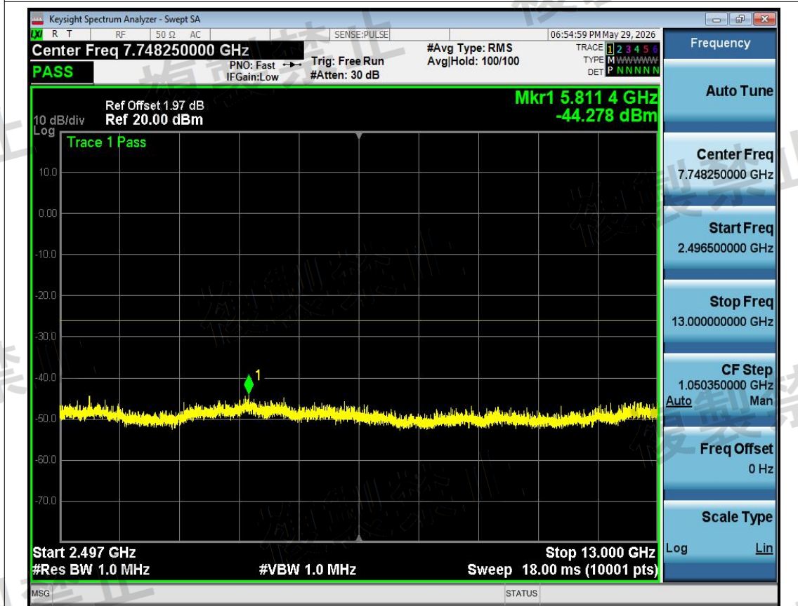
Tx. Spurious NVNT BLE 1M 2440MHz Ant1 @ 2496.5MHz-13000MHz
