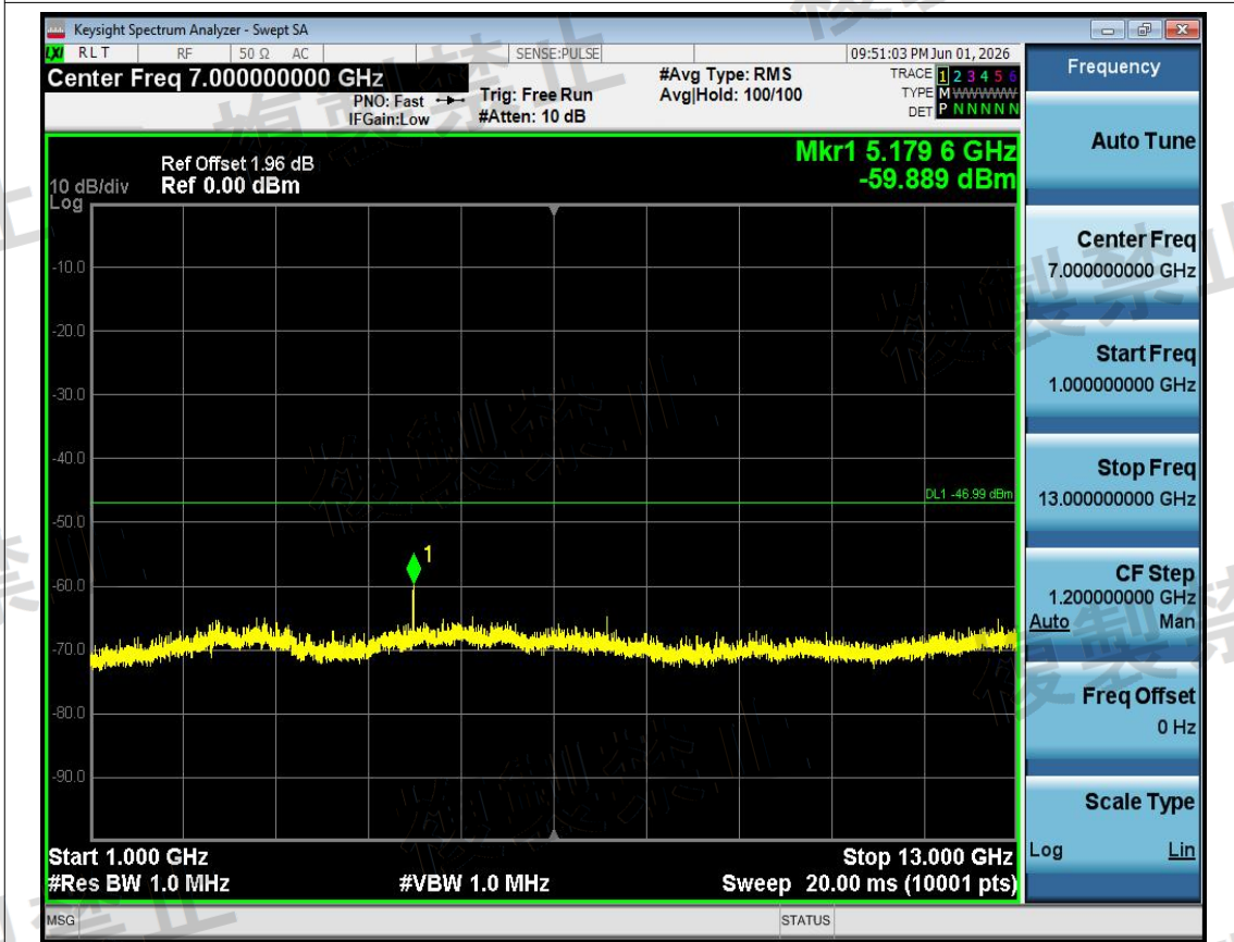
Rx. Spurious NVNT BLE 1M 2480MHz Ant1 @ 1000MHz-13000MHz
