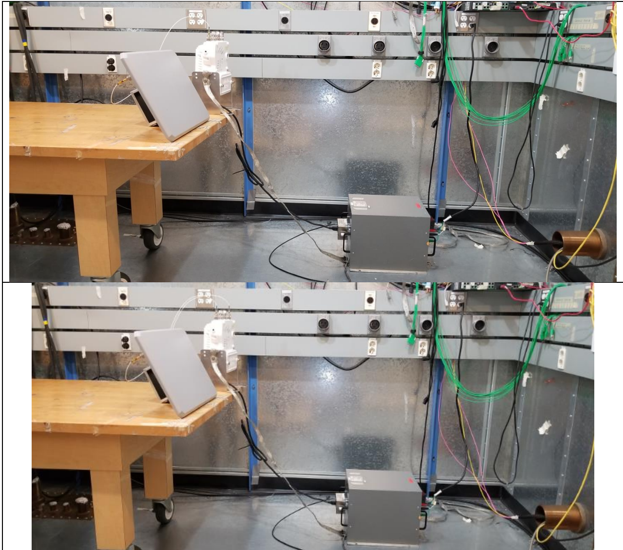
Title: Conducted Emissions 150KHz-30MHz – Test Setup
