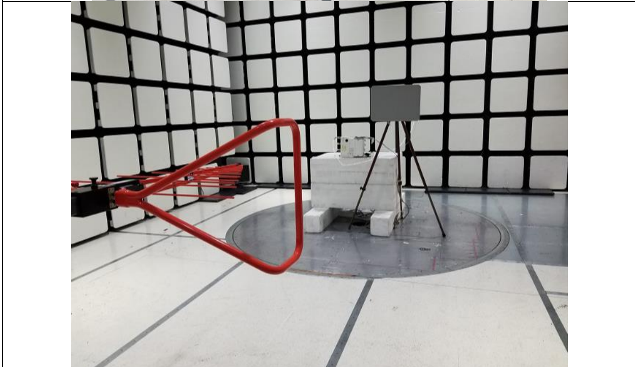
Title: Radiated Spurious Emissions 30MHz-1GHz – Test Setup
