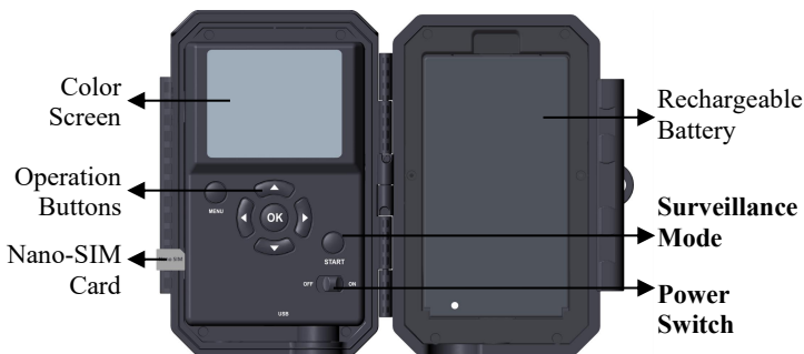
Figure 4: Inside View and Preinstalled SIM card
