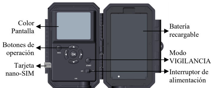
Figura 4: Inside view and pre-installed SIM card
