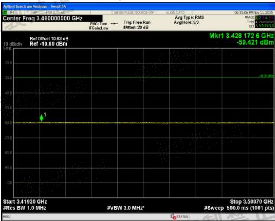
Band1(15L) QAM16 BW=15MHz Channel=18110 RB Size=1 Position=#0 Range3400 MHz-3419.3 MHz
