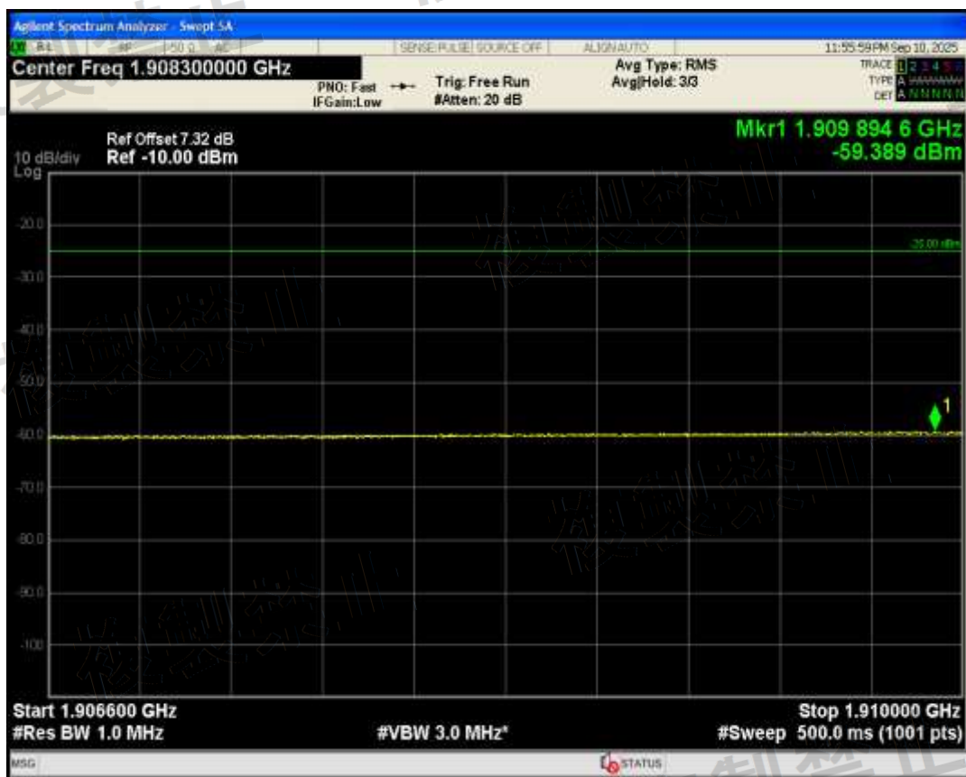
Band1(15H) QAM16 BW=15MHz Channel=18525 RB Size=75 Position=#0 Range1910 MHz-1915.7 MHz
