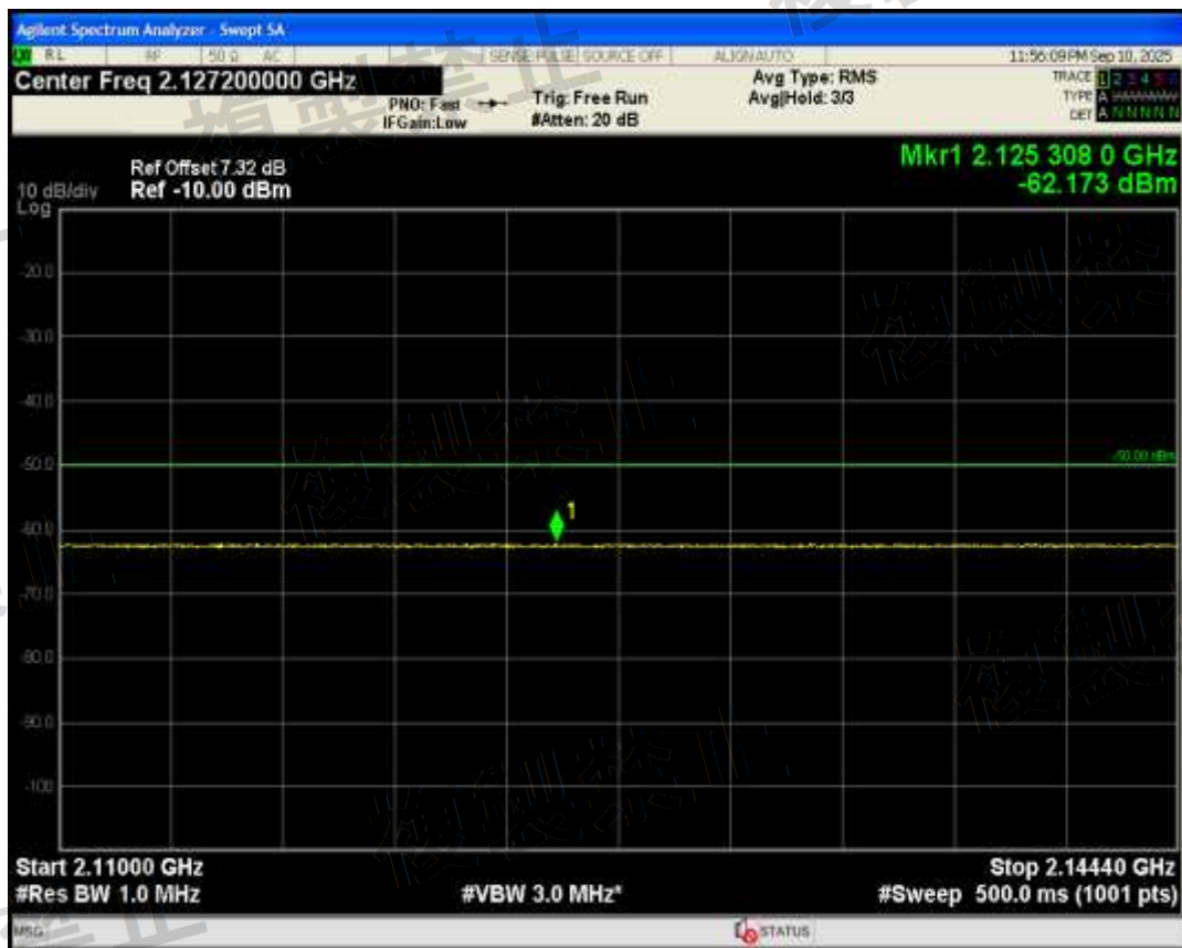
Band1(15H) QAM16 BW=15MHz Channel=18525 RB Size=75 Position=#0 Range=2144.4 MHz-2170 MHz
