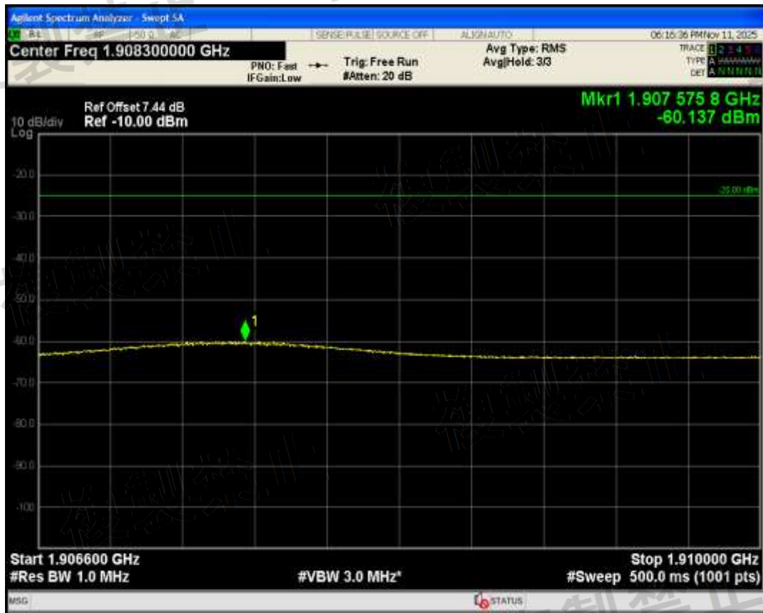
Band1(15L) QPSK BW=15MHz Channel=18075 RB Size=1 Position=#0 Range1910 MHz-1915.7 MHz
