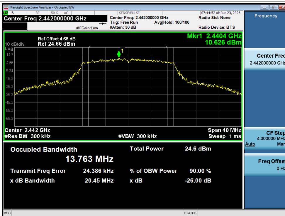
Spreading Bandwidth NVNT g 2442MHz Ant1
