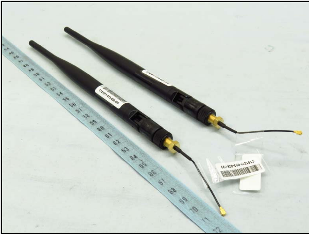
Dipole antenna, model: AOA-160-221050-000000
