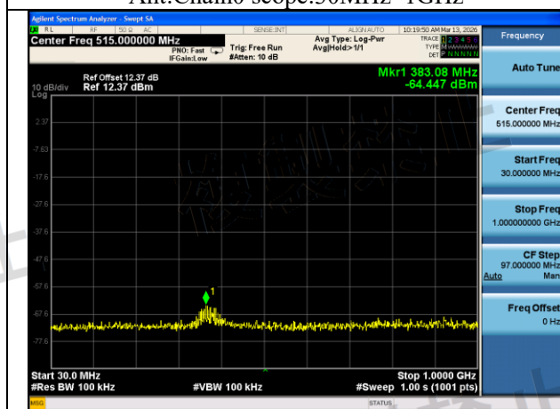
Mode:802.11ac VHT80 Frequency:5690MHz Ant:Chain0 scope:30MHz~1GHz
