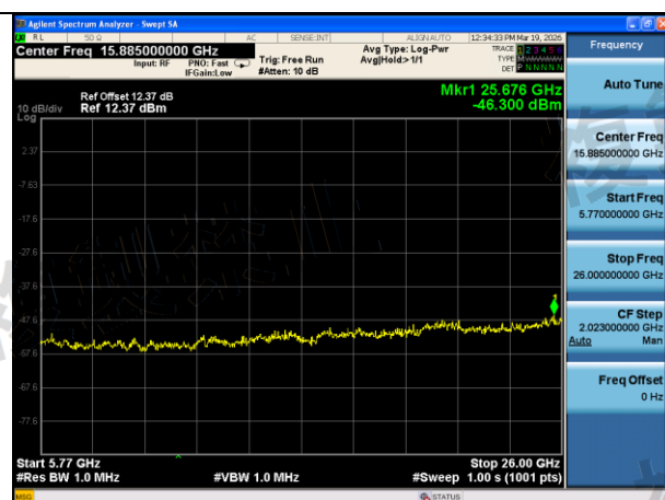
Mode:802.11n HT40 Frequency:5630MHz Ant:Chain0 scope:5770MHz~26GHz
