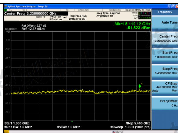
Mode:802.11n HT20 Frequency:5620MHz Ant:Chain1 scope:1GHz~5460MHz
