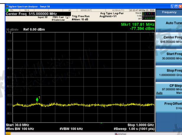
Mode:802.11n HT20 Frequency:5620MHz Ant:Chain1 scope:30MHz~1GHz
