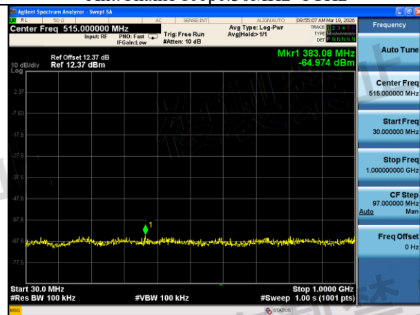
Mode:802.11ax HE20 Frequency:5720MHz Ant:Chain1 scope:30MHz~1GHz
