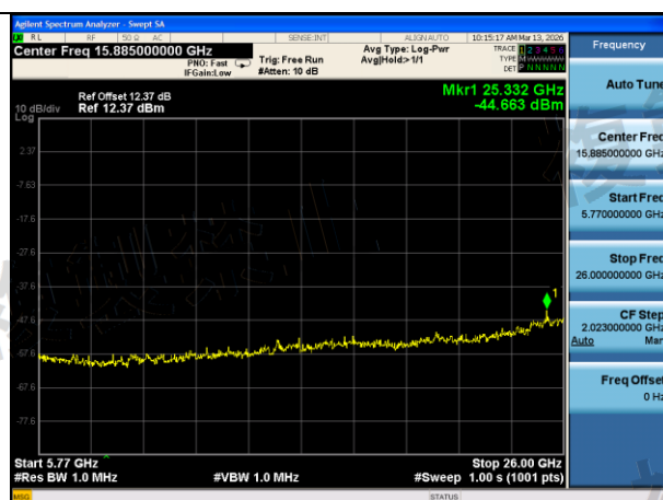
Mode:802.11ac VHT80 Frequency:5610MHz Ant:Chain0 scope:5770MHz~26GHz
