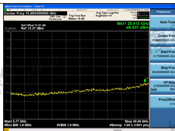
Mode:802.11ax HE40 Frequency:5630MHz Ant:Chain0 scope:5770MHz~26GHz
