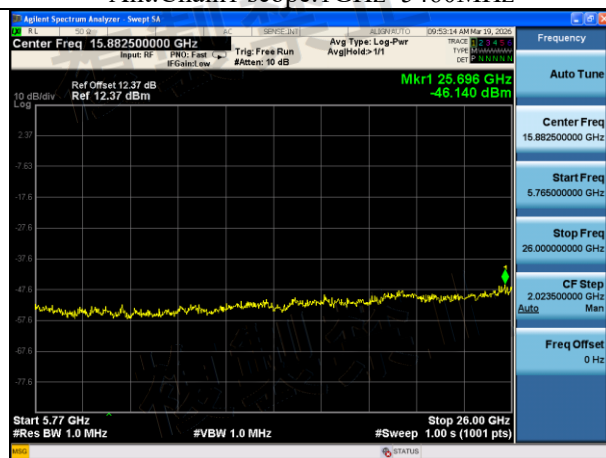
Mode:802.11ax HE20 Frequency:5500MHz Ant:Chain1 scope:5765MHz~26GHz
