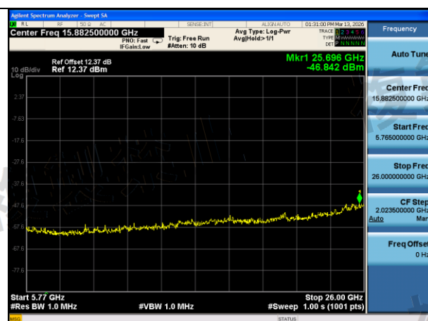
Mode:802.11n HT20 Frequency:5620MHz Ant:Chain0 scope:5765MHz~26GHz
