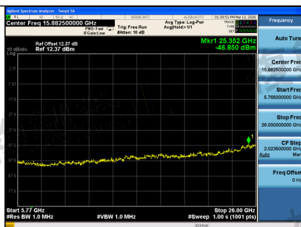
Mode:802.11ac VHT20 Frequency:5620MHz Ant:Chain0 scope:5765MHz~26GHz
