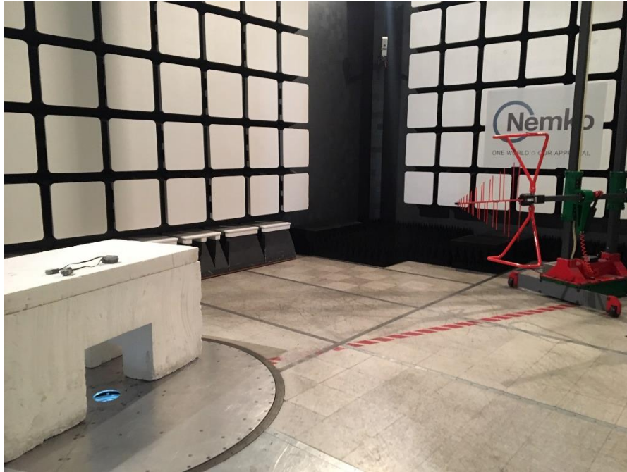
Figure 8.3-19: Radiated spurious emissions setup photo – below 1 GHz
