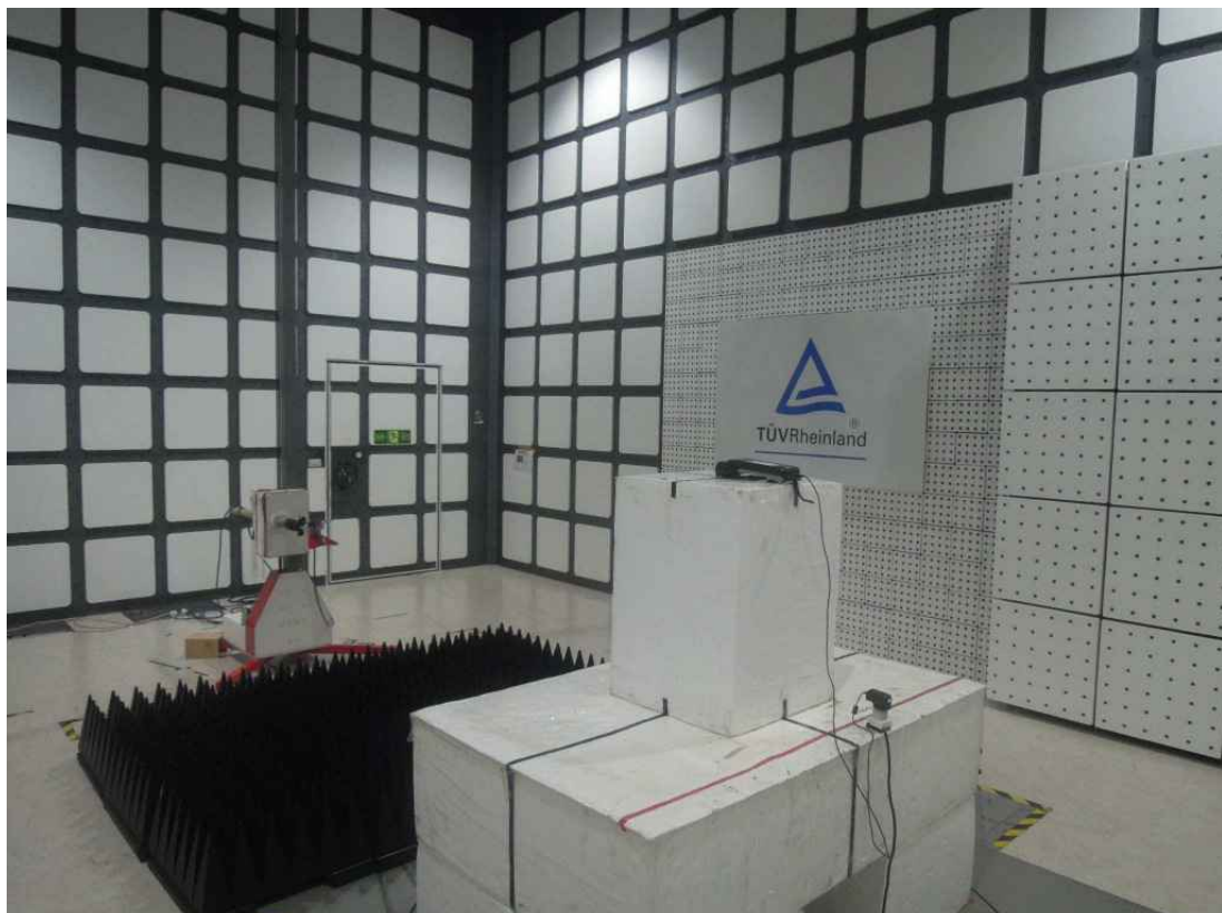
Photograph 5: Set-up for Spurious Emissions (Back View 3)
