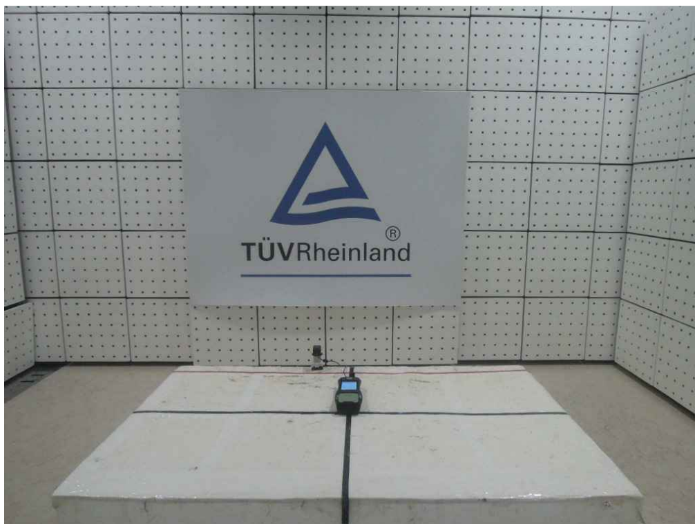
Photograph 1: Set-up for Spurious Emissions (Front View 1)
