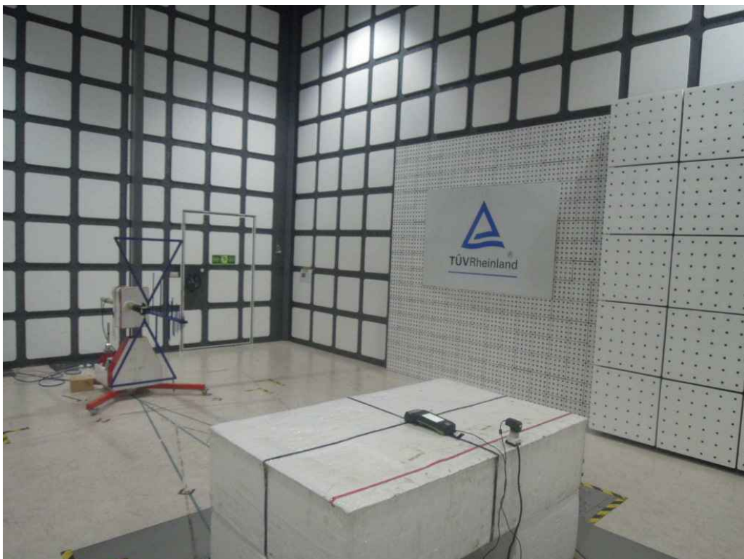
Photograph 3: Set-up for Spurious Emissions (Back View 1)
