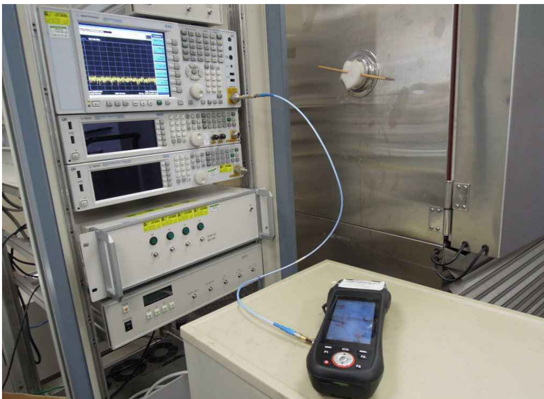
Photograph 7: Set-up for Conducted testing
