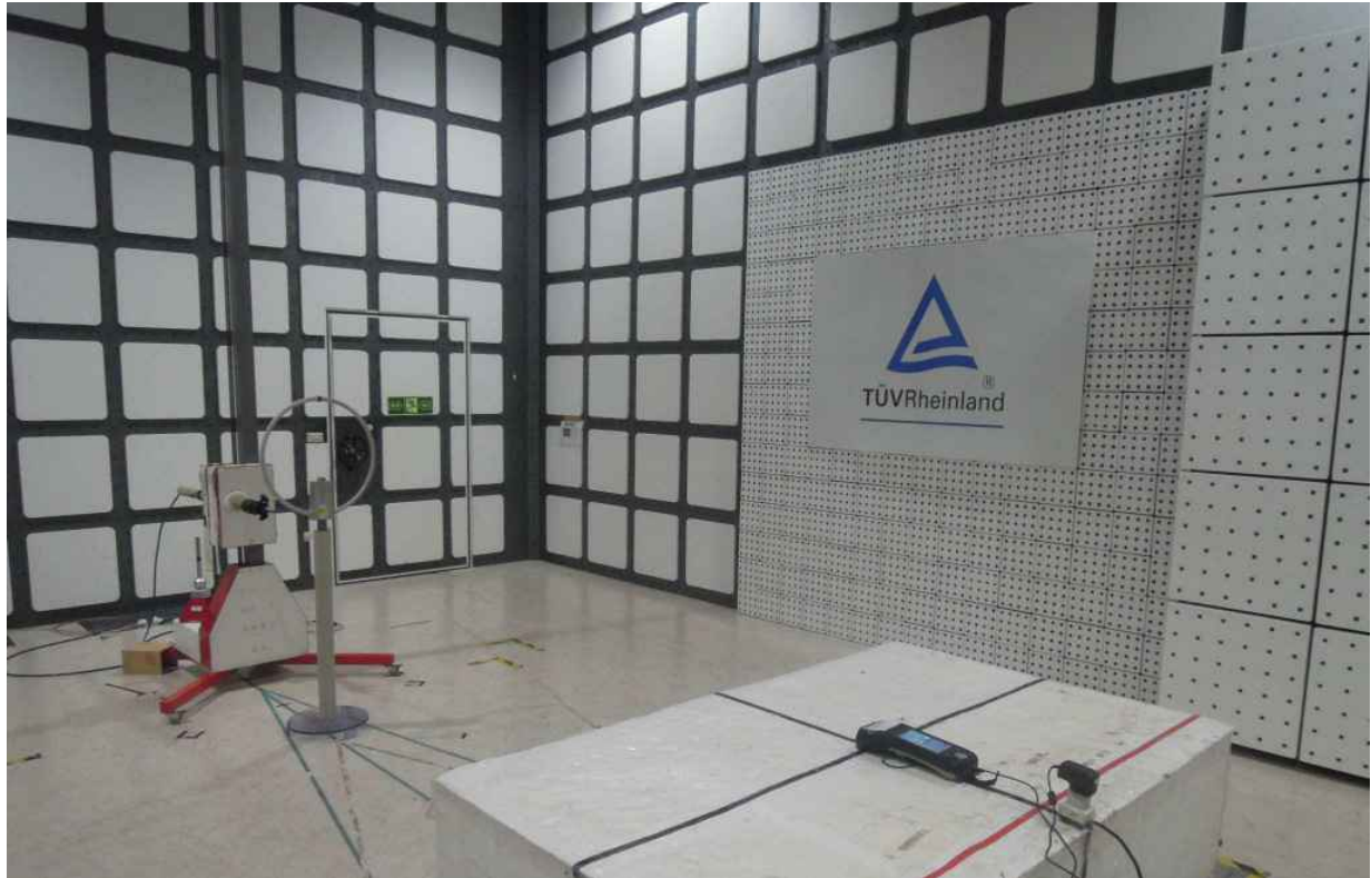
Photograph 5: Set-up for Spurious Emissions (Back View 3)
