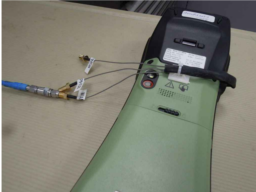
Photograph 9: Set-up for Mains Conducted testing (Back View)
