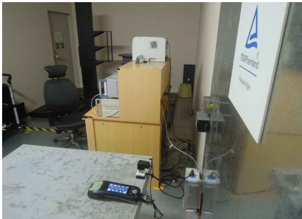
Photograph 9: Set-up for Mains Conducted testing (Back View)
