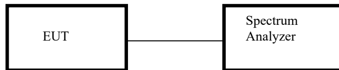
Figure 10. Spurious Emissions Test Configuration
