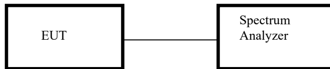
Figure 24. Secondary Emissions (Spurious Emission of Receiver) Test Configuration
