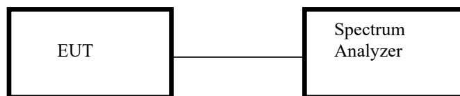
Figure 7. Occupied Bandwidth and Spread Spectrum Bandwidth Test Configuration
