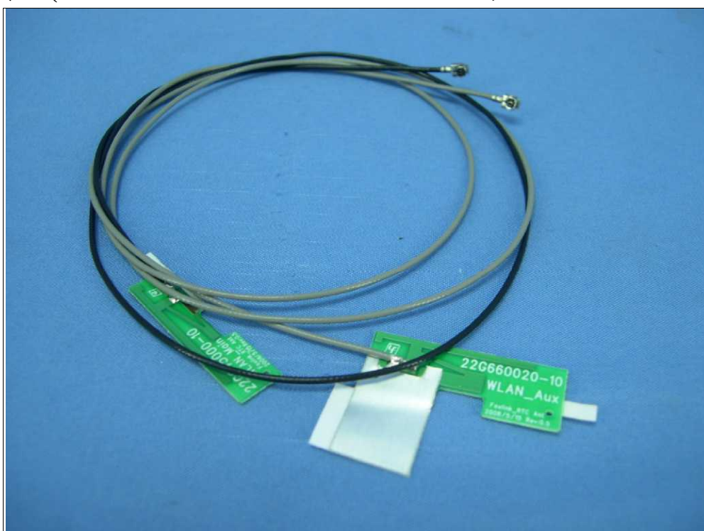
天線 71 (Brand: Foxlink / Model: A40/A41-L 22G645000-10, A40/A41-R 22G660020-10)
