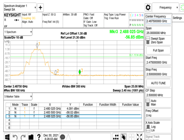
Spurious Emission_BLE 1M_LowCH00-2402MHz
