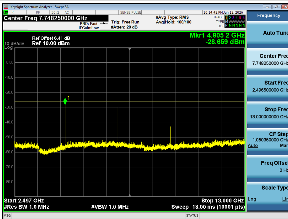
Tx. Spurious NVNT 1-DH5 2402MHz Ant1 @ 2496.5MHz-13000MHz
