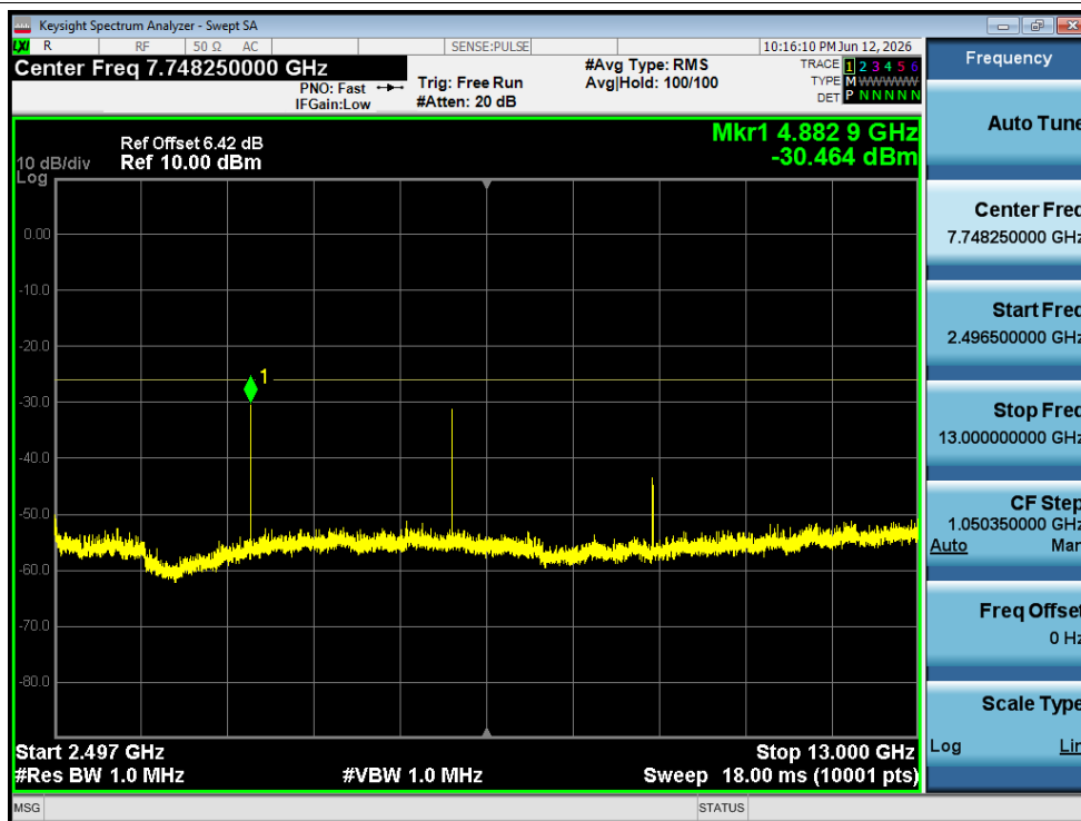
Tx. Spurious NVNT 1-DH5 2441MHz Ant1 @ 2496.5MHz-13000MHz
