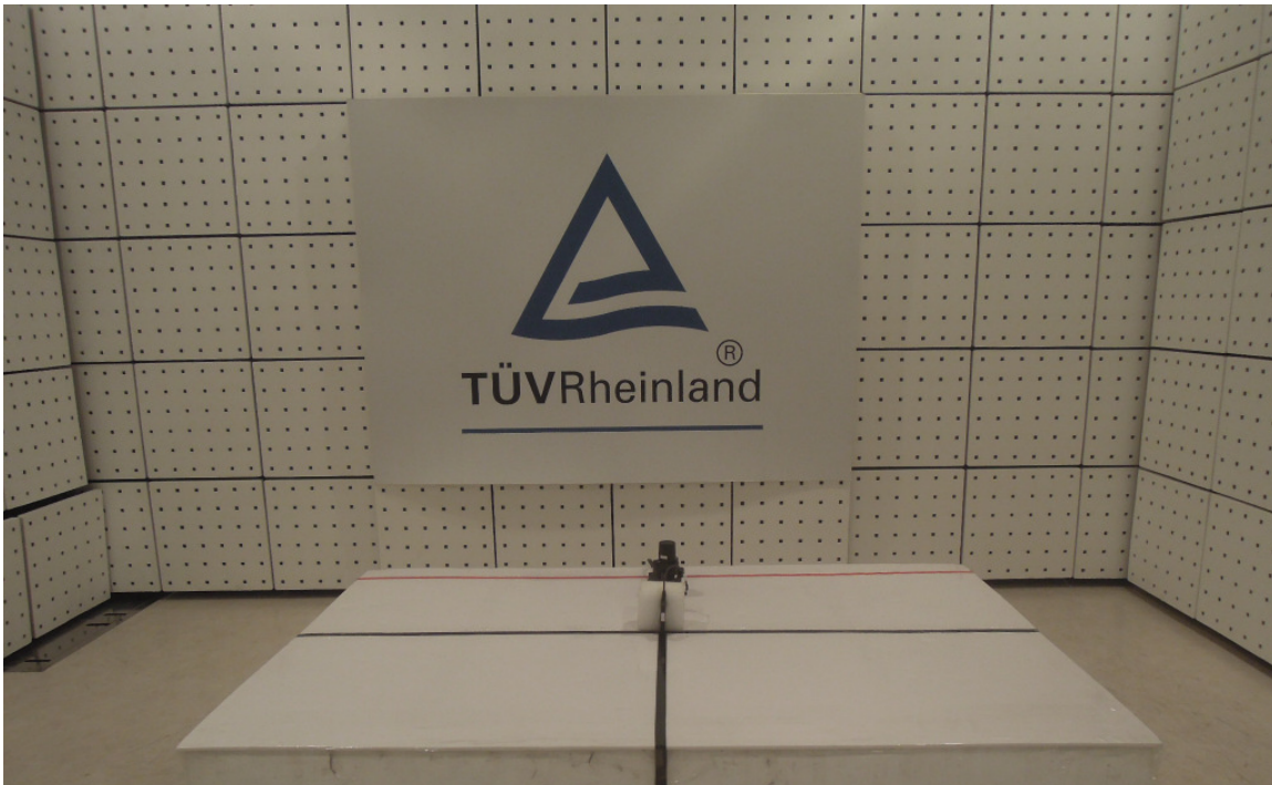
Photograph 1: Set-up for Spurious Emissions (Front View)
