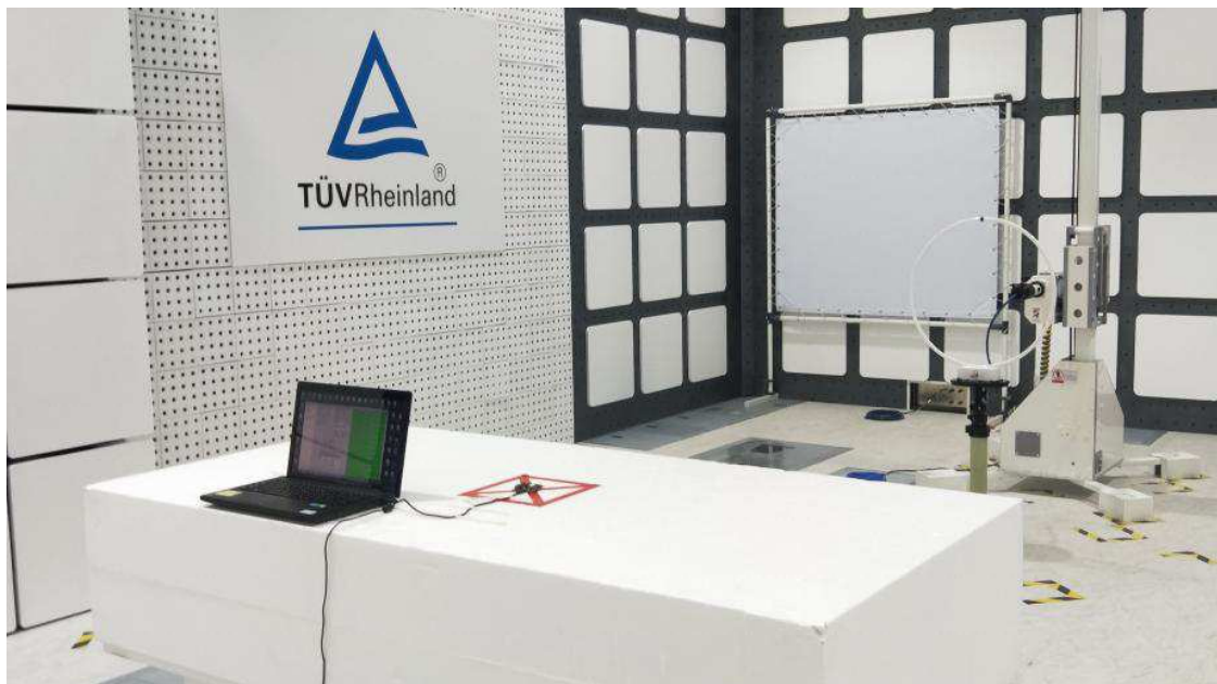
Photograph 4: Set-up for Spurious Emissions (Back View 2)
