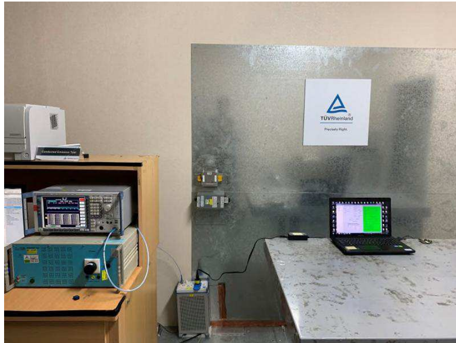
Photograph 9: Set-up for Mains Conducted Emissions
