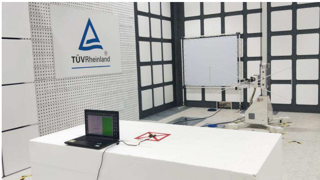
Photograph 6: Set-up for Spurious Emissions (Back View 4)
