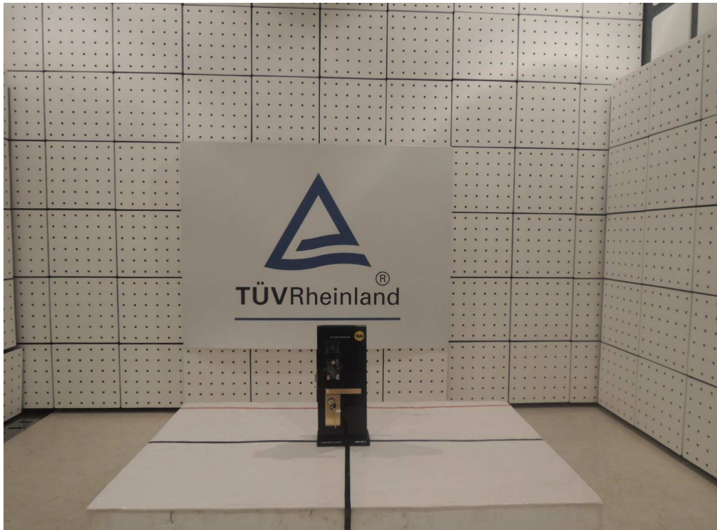
Photograph 2: Set-up for Radiated Emissions (Back View 1)
