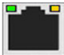
Fig. 4: RJ45 LEDs Ethernet RJ45 LED Indicators
