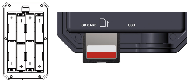
Figure 5: Installation of batteries and SD card
