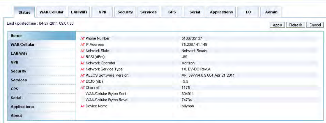
Figure 3-1: ACEmanager: Status - Home
