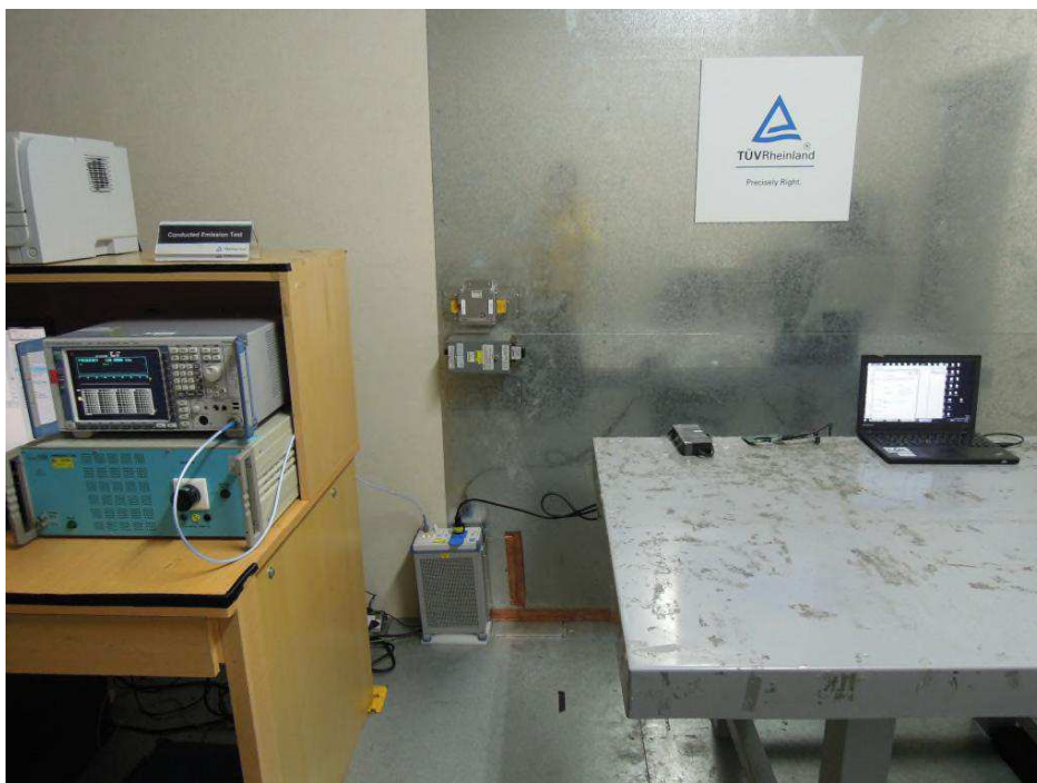
Photograph 11: Set-up for Mains Conducted testing Front, Z10NE030
