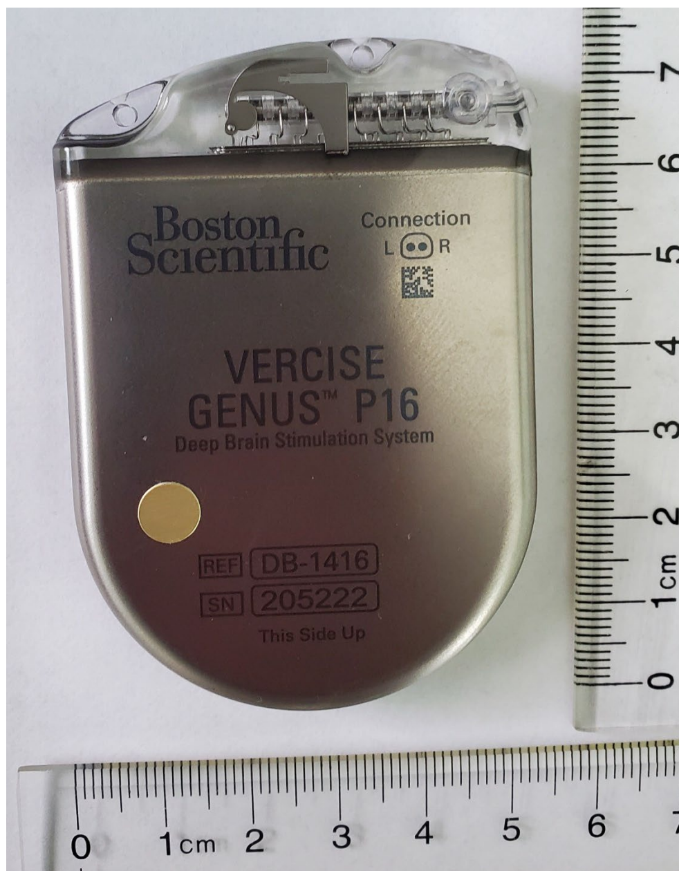
Figure 1: 16 Electrode Blink IPG External Photo – Frontside
