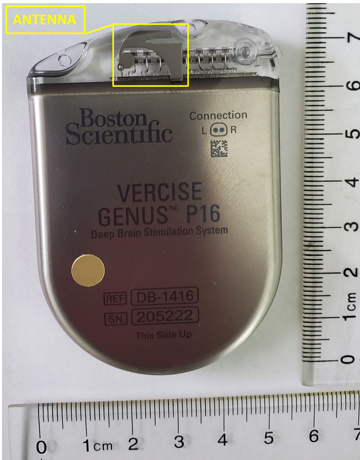
Figure 2: 16 Electrode Blink IPG External Photo – Frontside (antenna outlined)
