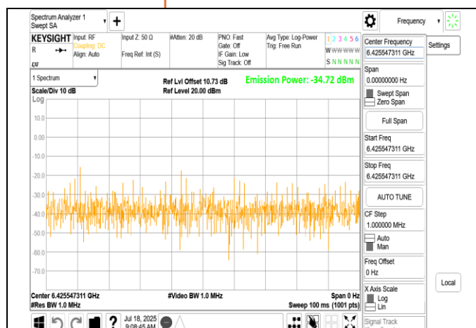
LPI 802.11be 160MHz Chain0 6345MHz Range3 Sample
