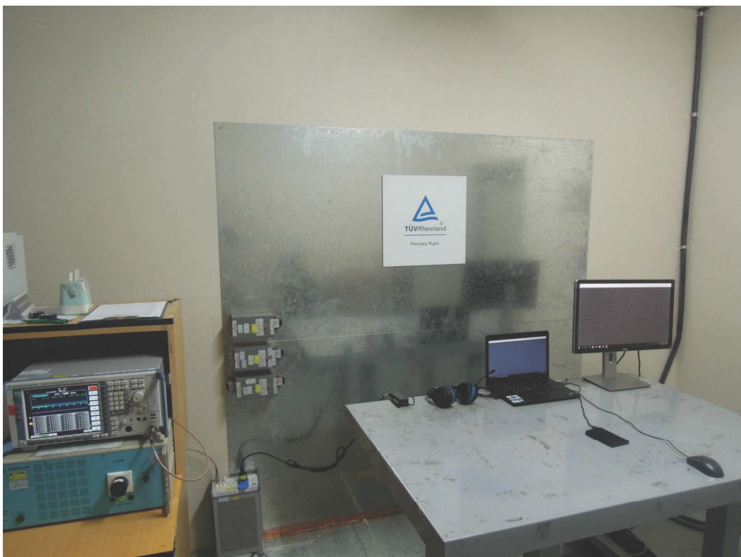
Photograph 6: Set-up for Mains Conducted testing (Front)
