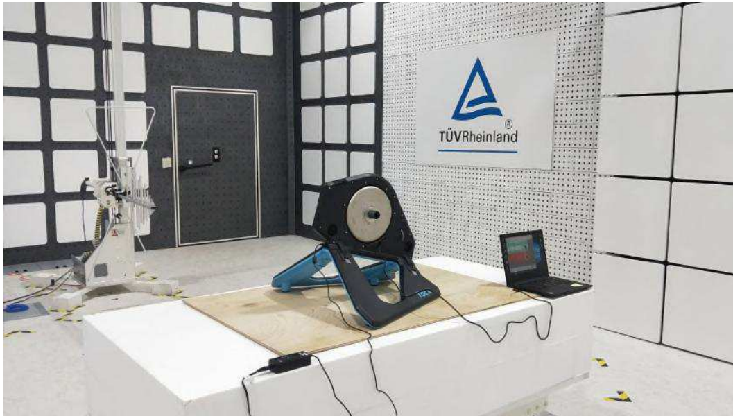
Photograph 3: Set-up for Spurious Emissions (Back View 1)
