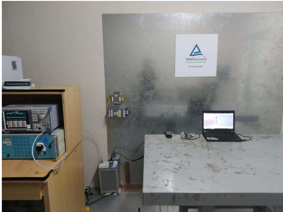
Photograph 9: Set-up for AC Mains (View 1)
