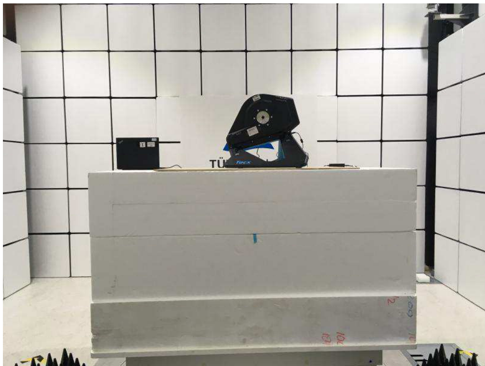
Photograph 2: Set-up for Spurious Emissions (Front View 2)
