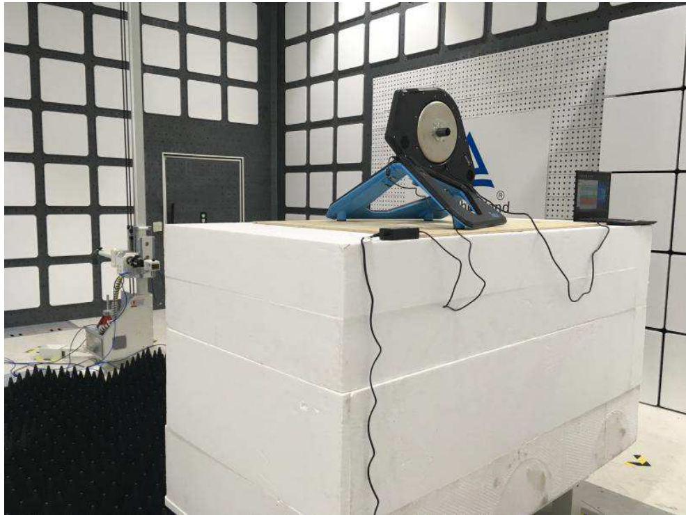
Photograph 5: Set-up for Spurious Emissions (Back View 3)
