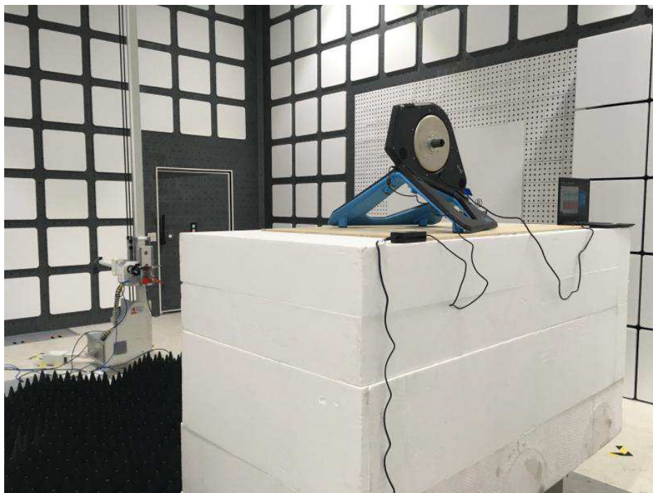
Photograph 6: Set-up for Spurious Emissions (Back View 4)
