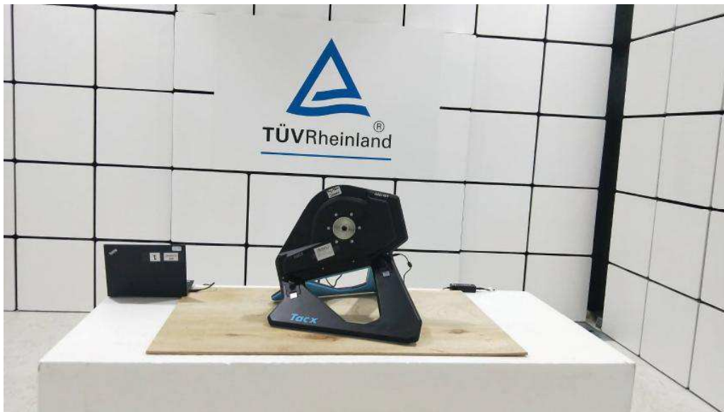
Photograph 1: Set-up for Spurious Emissions (Front View 1)
