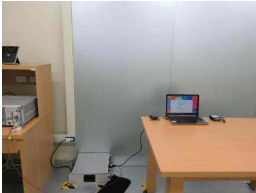
Photograph 7: Set-up for AC Mains (Front View)
