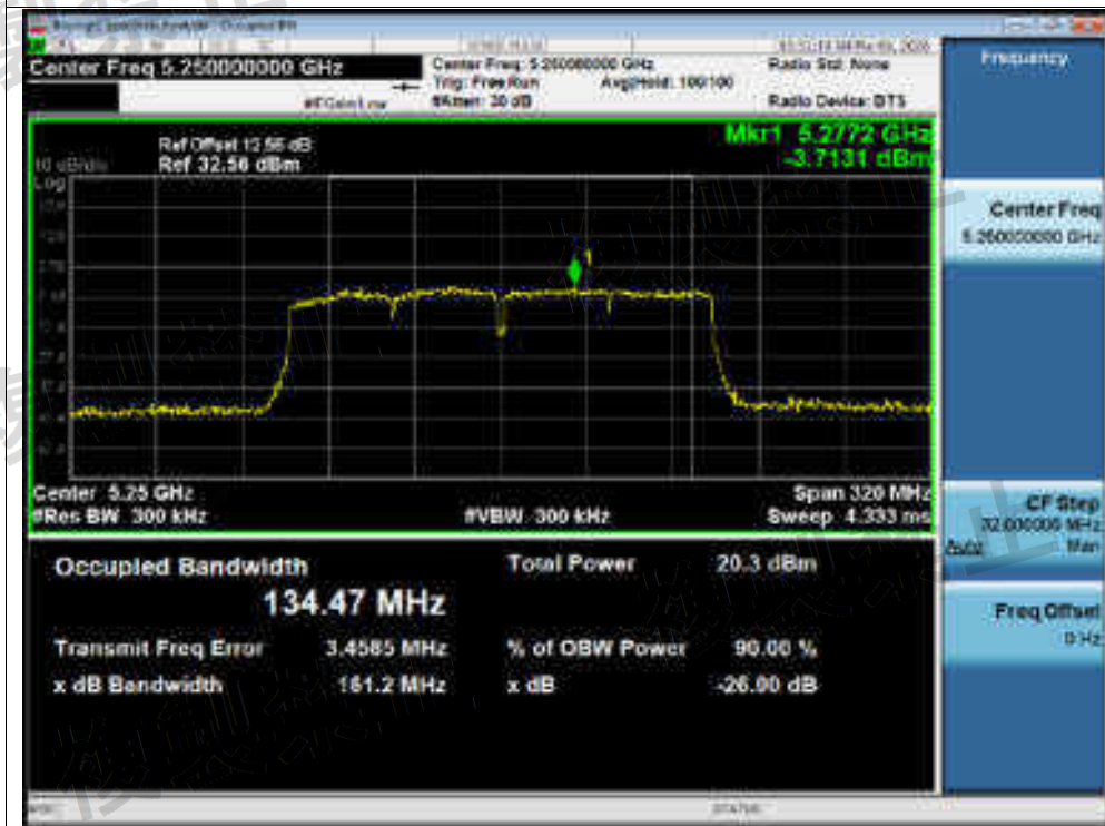
Spreading Bandwidth NVNT ac160 5250MHz Ant2
