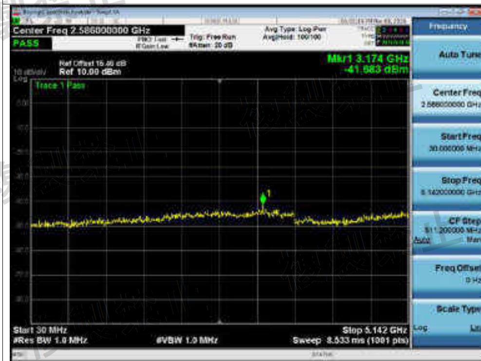
Tx. Spurious NVNT ax20 5240MHz Ant1 @ 5142MHz-5150MHz
