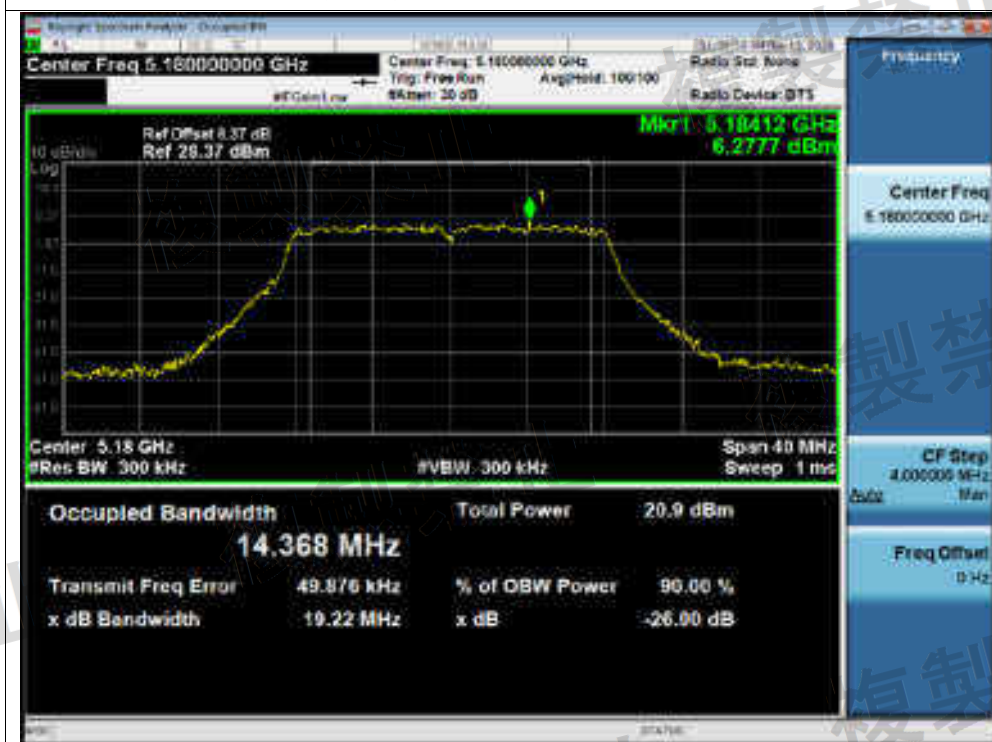
Spreading Bandwidth NVNT a 5180MHz Ant2
