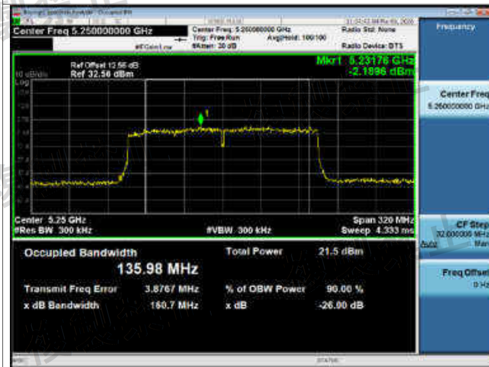
Spreading Bandwidth NVNT ax160 5250MHz Ant2
