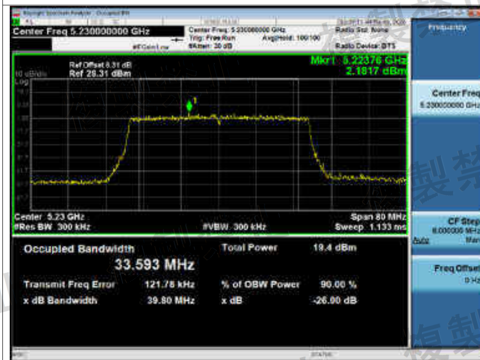
Spreading Bandwidth NVNT ax40 5230MHz Ant2
