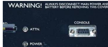
Figure 7. Internal RS-232 connector for the console
