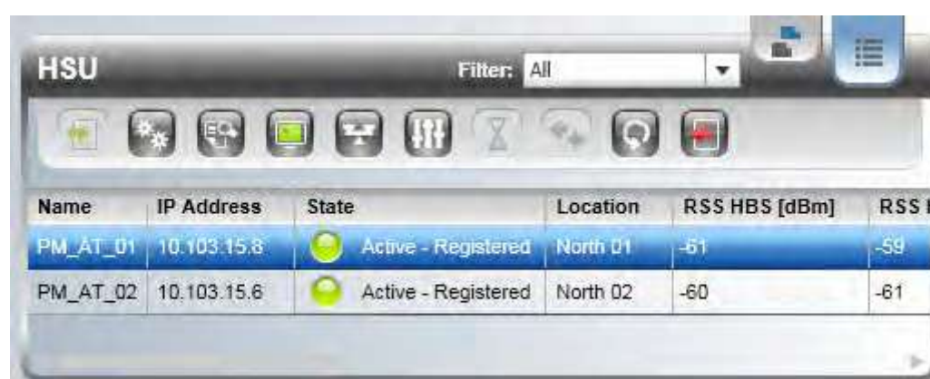
Figure 4-16: HSU display - detail. Scroll right for more fields
