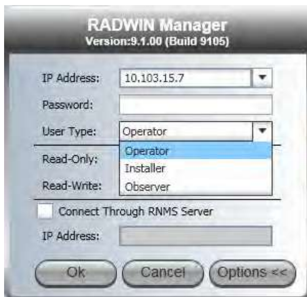
Figure 4-4: Log on window exposing the user types.
