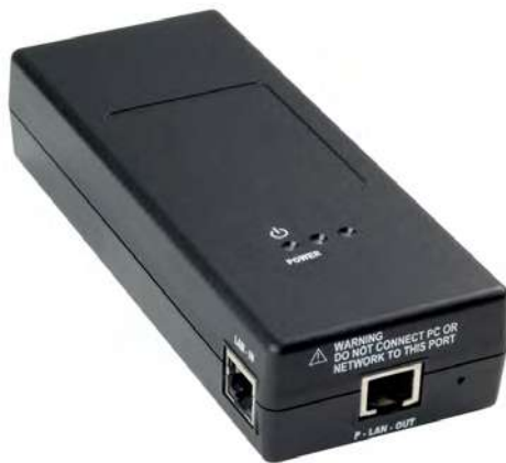
Figure 3-4: Basic PoE device - showing the radio Ethernet port
