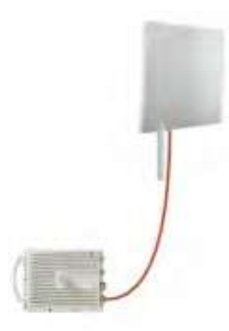
Figure 8-7: Incorrectly mounted ODU (No “water nose”)
