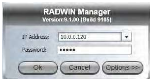
Figure 5-1: Logging on with factory default IP address
