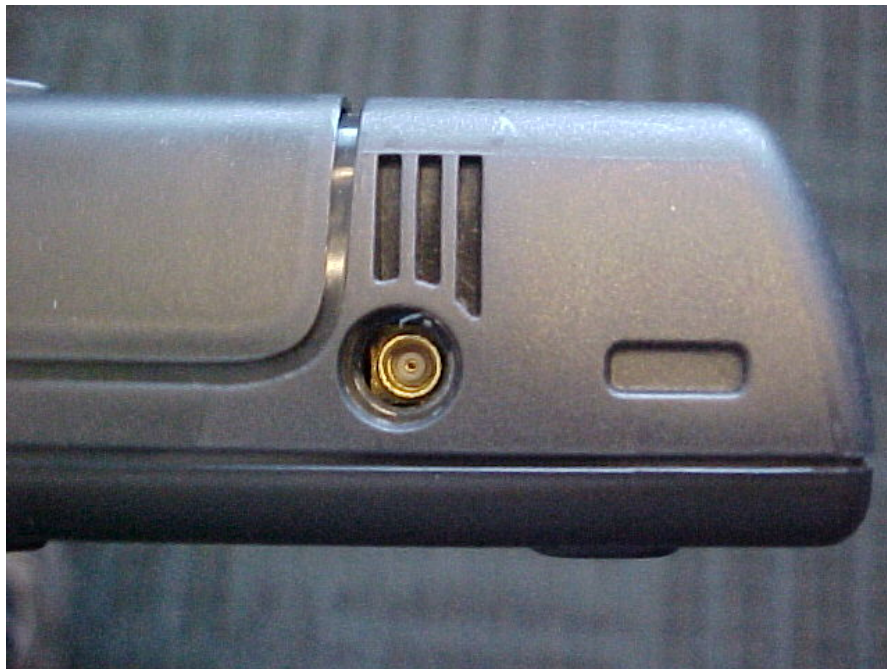
Figure 18. External GPS Antenna RF Connector.
